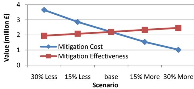
Figure 7-39 Sensitivity of the value of insulating lines to mitigation cost and effectiveness
