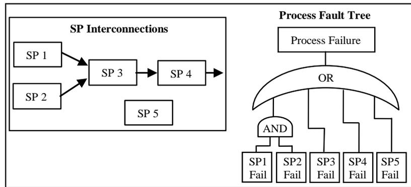
Figure 5-38 Fault tree analysis on a general process
