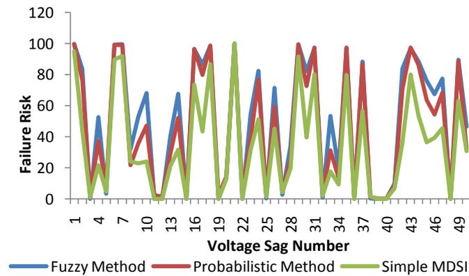
Figure 5-27 Failure risk of PLC with moderate sensitivity for 50 random voltage sag events
