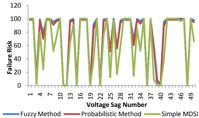
Figure 5-24 Failure risk of ASD with high sensitivity for 50 random voltage sag events
