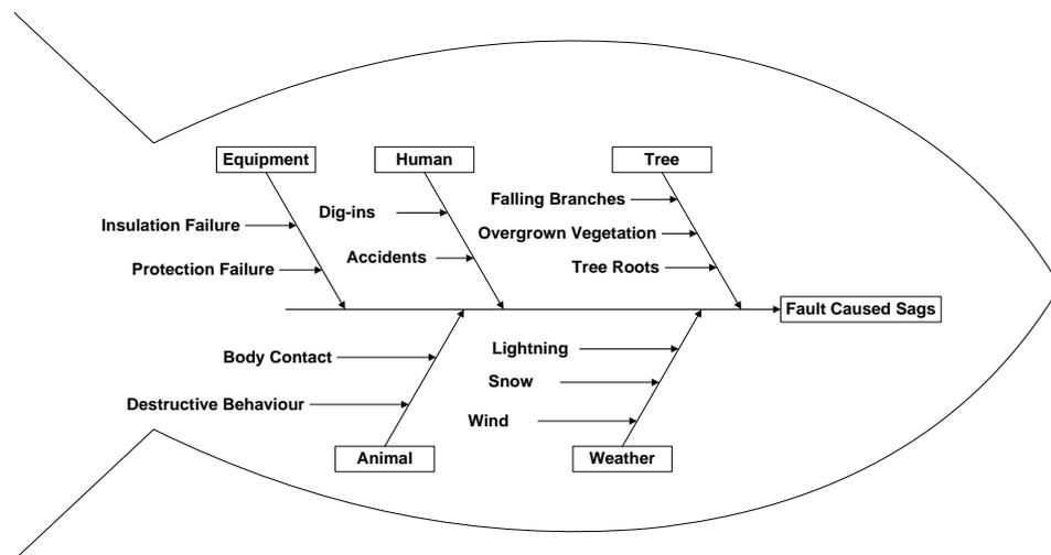
Figure 6-7 The causes of fault-caused sags and interruptions
