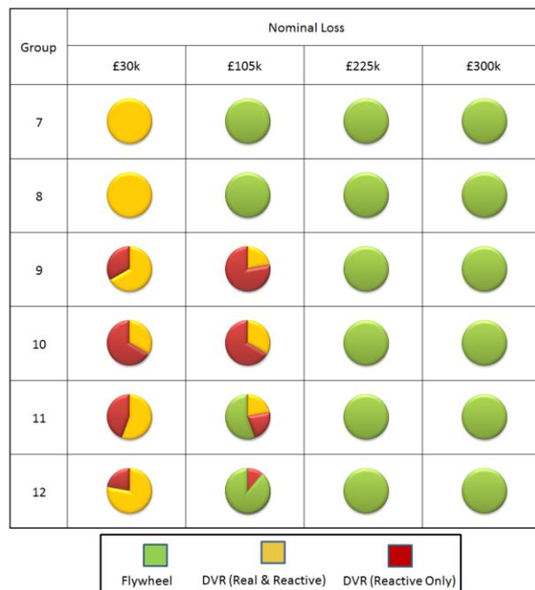
Figure 7-19 Optimal power injecting device for process Group 7 to 12
