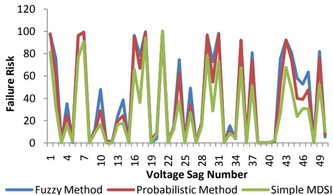
Figure 5-19 Failure risk of PC with moderate sensitivity for 50 random voltage sag events
