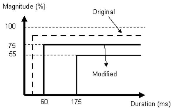
Figure 6-16 Modification of ASD tolerance curve after improvement
