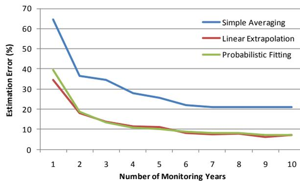
Figure 5-54 Average error in voltage sag profile estimation.
