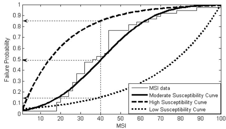
Figure 5-17 Probabilistic model representing magnitude failure probability
