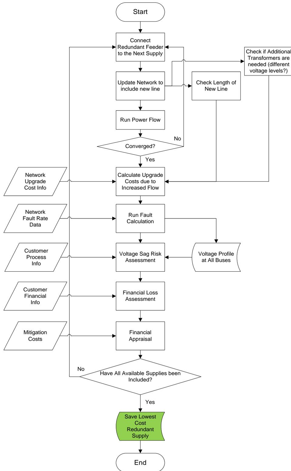
Figure 7-28 Optimal redundant supply assessment flow chart
