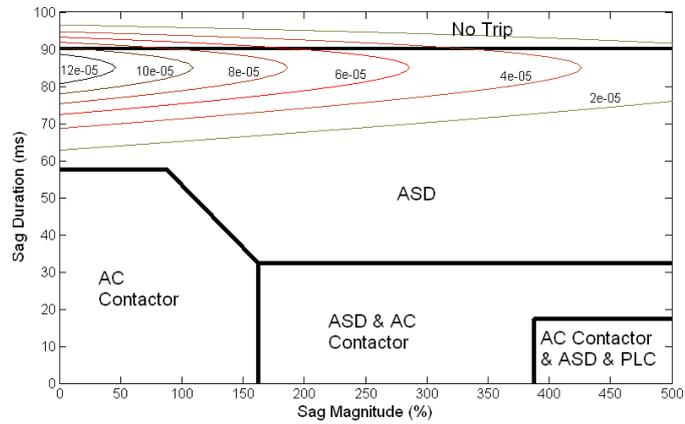
Figure 6-15 Determining of the most vulnerable equipment
