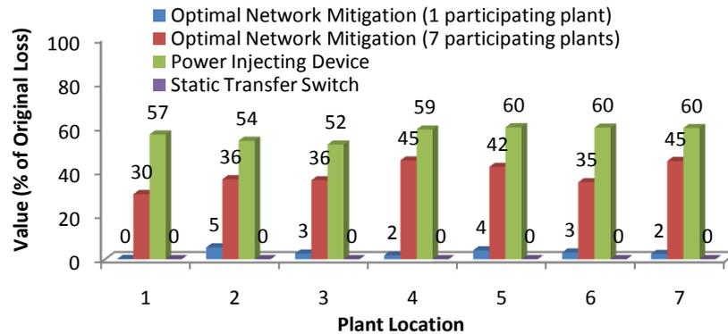
Figure 7-89 The value of optimal network fault reduction with seven participating type-37 plants
