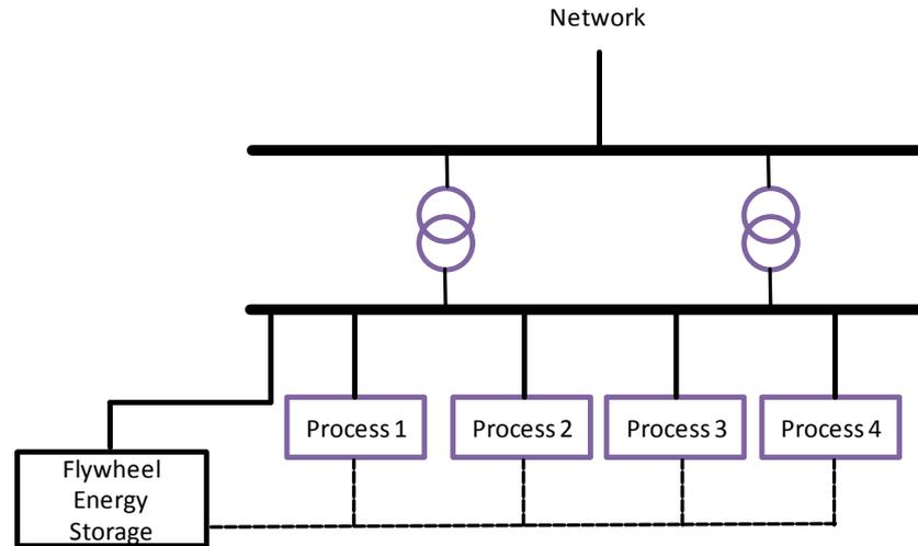
Figure 6-3 Flywheel energy storage at customer plant
