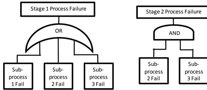
Figure 5-62 Process cycle stage 1 and stage 2 fault trees
