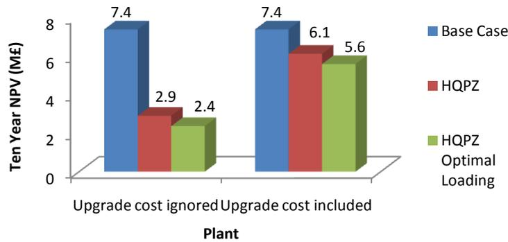
Figure 8-25 Total post mitigation losses with best mitigation scheme (30% transmission sags)
