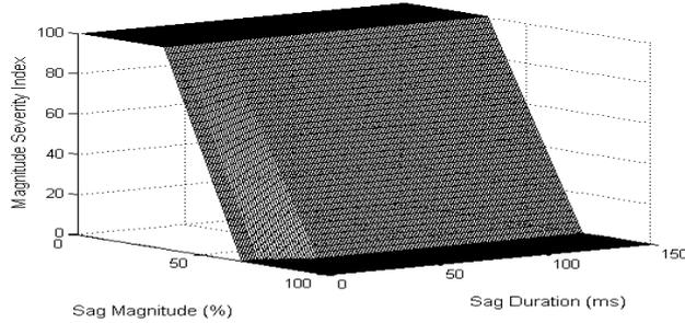
Figure 5-11 MSI conversion graph of AC contactor
