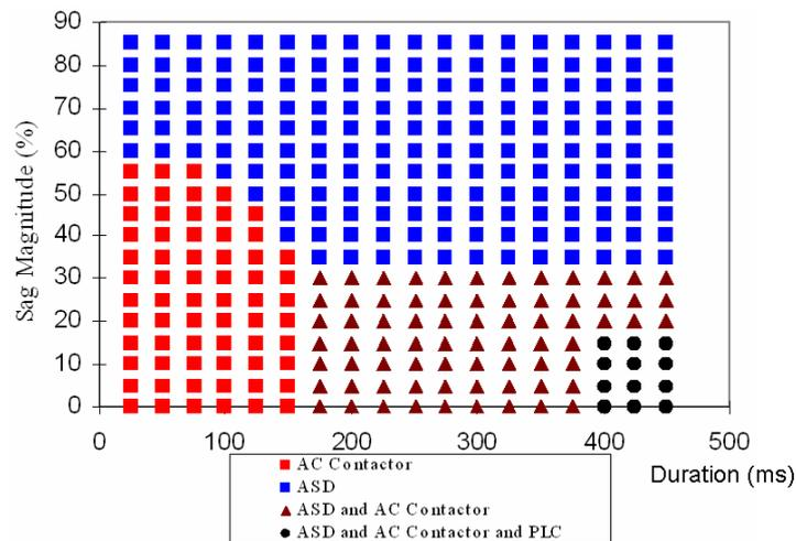
Figure 6-13 The weakest link in the process.
