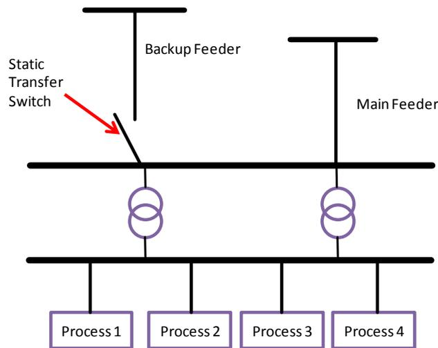
Figure 6-6 Static transfer switch at customer plant
