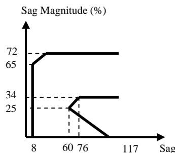
Figure 5-10 Boundaries of AC contactor voltage tolerance. Adopted from [33]
