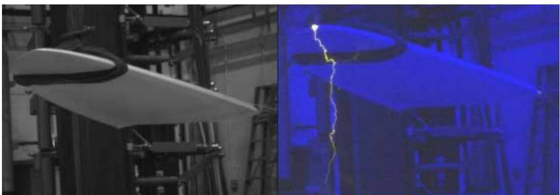
Figure 7-17 Positive Streamers from Tip on RCS Blade at 600kV in Position A (left figure to show blade in day light for comparison)
