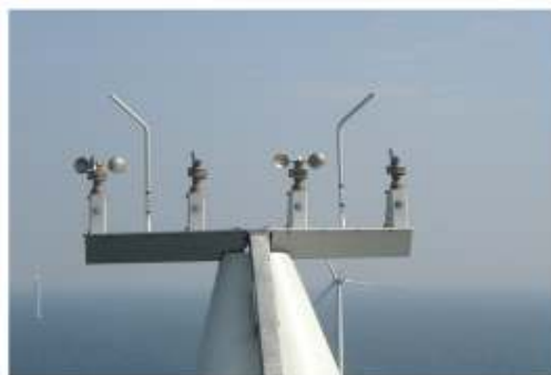
Figure 5-5 Wind Instruments Protected by Lightning Rods
