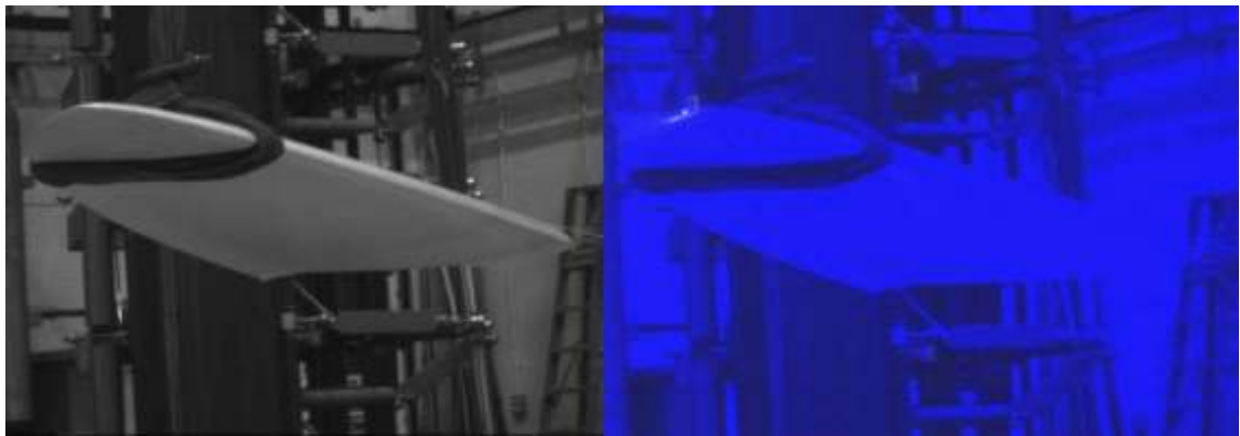
Figure 7-18 Negative Streamers from Tip on RCS Blade at 1050kV Position A (left figure to show blade in day light for comparison)
