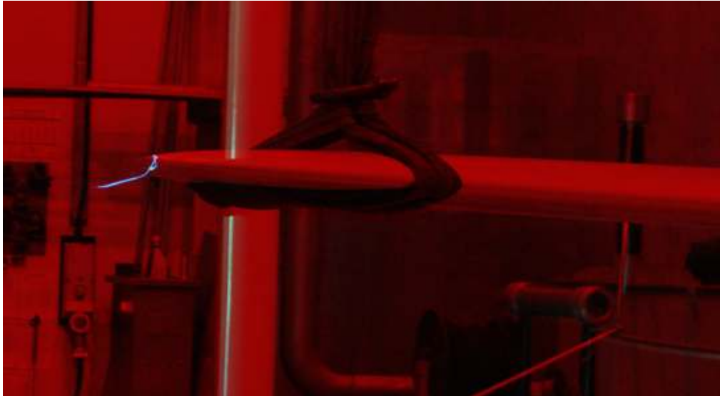
Figure 7-19 Negative Streamers from Tip on RCS Blade at 1050kV (Position A) from conventional camera
