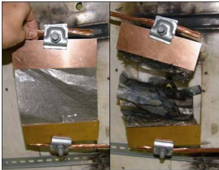
Figure 6-13 Current Conduction Test (50g/m 2 without resin, before and after test)
