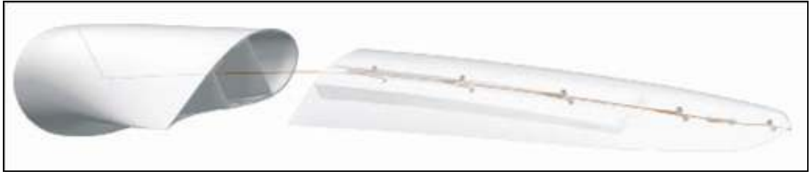
Figure 3-6 Receptor/Down Conductor based lightning protection system [32]
