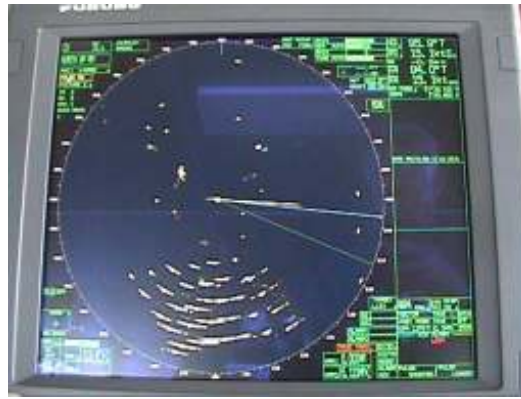
Figure 6-3 Target Spreading and Side Lobe Detection [70]
