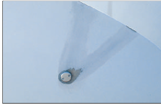
Figure 3-8 Tip receptor and erosion towards the edge of the blade
