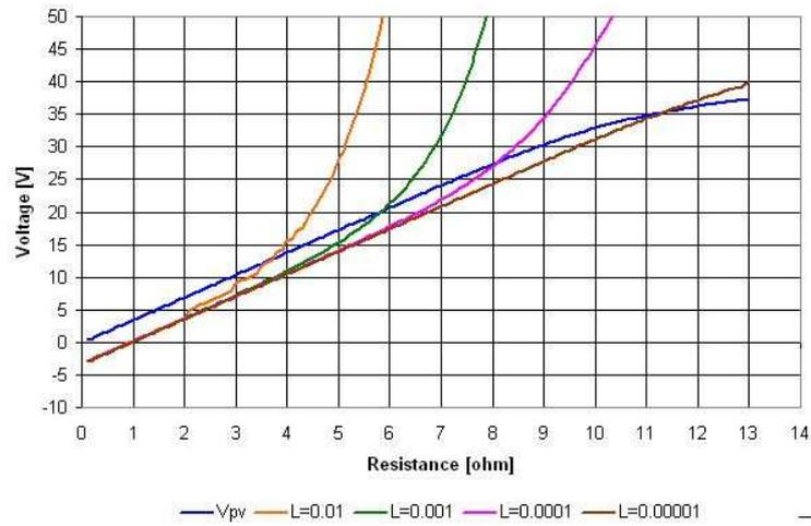
Figure 5-11: Variation of convergence limit with load resistance for different inductor values and output voltage of the photovoltaic panel ( $V_{pv}$ ) with load resistance
