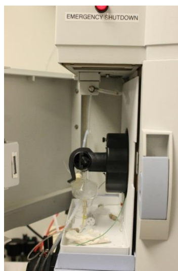
Figure 6.2 The pump and nebuliser that converts the liquid samples to aerosol
