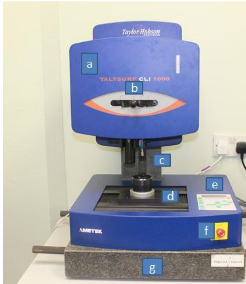
Figure 3.2 3D optical profilometer: (a) gauge cover, (b) gauge selection, (c) vertical Z slide, (d) horizontal X-Y slides, (e) remote control keypad, (f) emergency stop button, and (g) granite base and gantry
