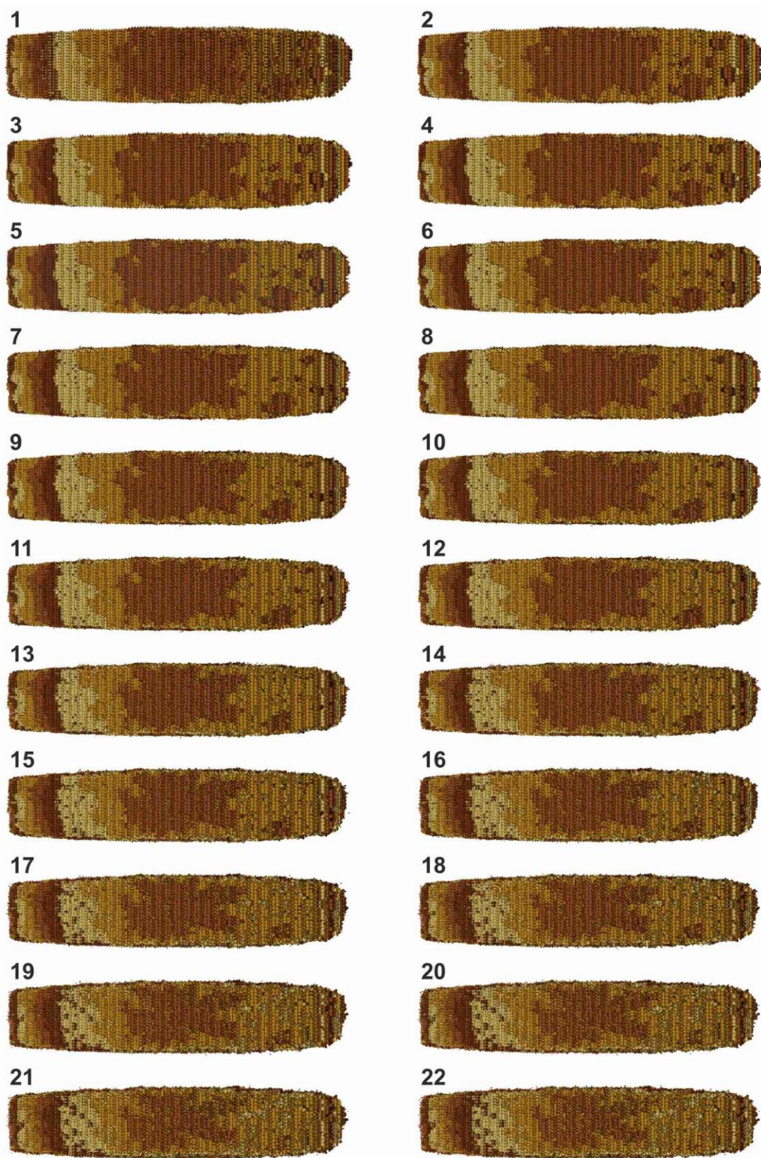
Figure 3.32. Subsequent images of IM-17 crystal dissolution simulation on (013) facet with \Delta\mu_{\text{eq}} = 9.7 and \Delta\mu for dissolution = 5. The simulation was set with \Delta U_s = 2 \text{ kcal mol}^{-1} . The (013) facet of the simulated crystal above is c.a. 0.04 \mu\text{m} \times 0.14 \mu\text{m} . The first image is the crystal before the dissolution started ( to be continued on the next page ).
