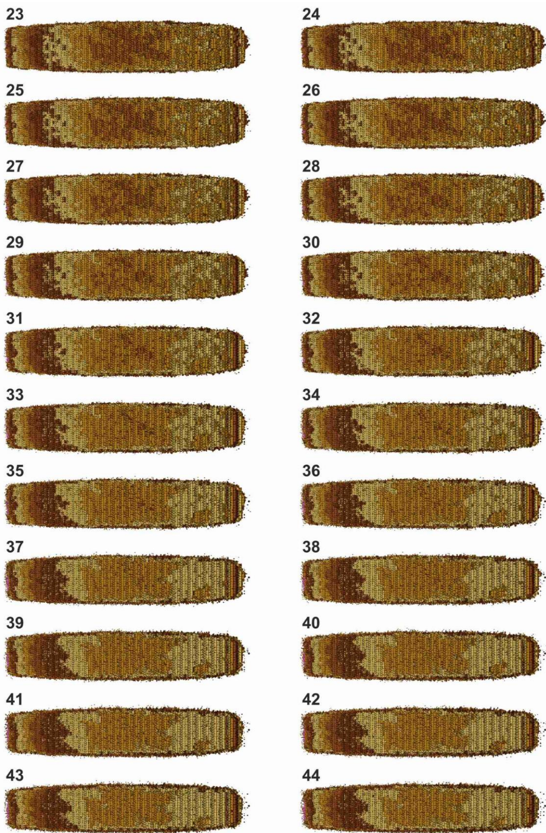
Figure 3.32 (continued). Subsequent images of IM-17 crystal dissolution simulation on (013) facet with \Delta\mu_{\text{eq}} = 9.7 and \Delta\mu for dissolution = 5. The simulation was set with \Delta U_s = 2 \text{ kcal mol}^{-1} . The (013) facet of the simulated crystal above is c.a. 0.04 \mu\text{m} \times 0.14 \mu\text{m} . The first image is the crystal before the dissolution started.
