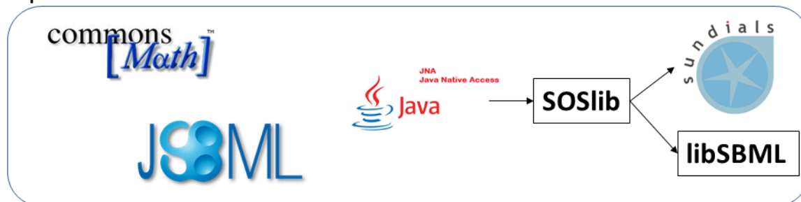
Figure 2.3: Architecture of GPaPe 2.0. The software is written in a modular nature, where each main function is written in separate packages in Java, such as the main ones for Model, Genetic Algorithm and Graphical User Interface (GUI). This allows for the software to be used via a command line interface (CLI) if preferred. In order for the software to work, three Java libraries (Apache Common Maths, JSBML, Java Native Access) and three C libraries (SBML Odesolver, SUNDIALS, libSBML) are required.
