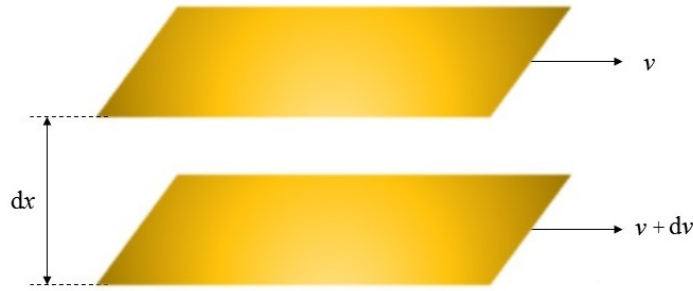
Figure 2.2.8. Viscosity as the friction forces between liquid layers.
