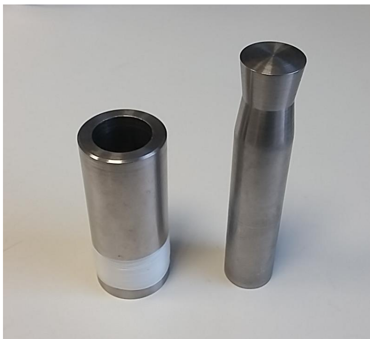
Figure 3.1: The stainless steel pestle and mortar used to crush each meteorite chip prior to freeze-thaw disaggregation. The mortar consists of two pieces, which were sealed with Teflon tape to ensure no fine dust could escape.
