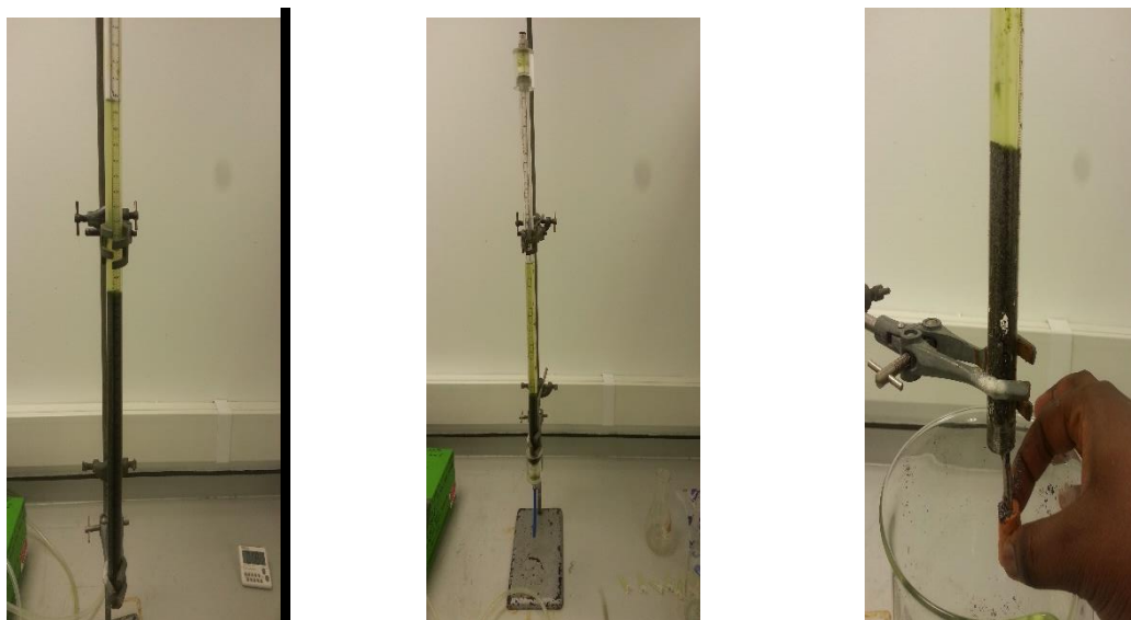
Figure 4:49: Pictorial image of bed blockage, showing that liquid above the bed is not able to pass downward through the column.
