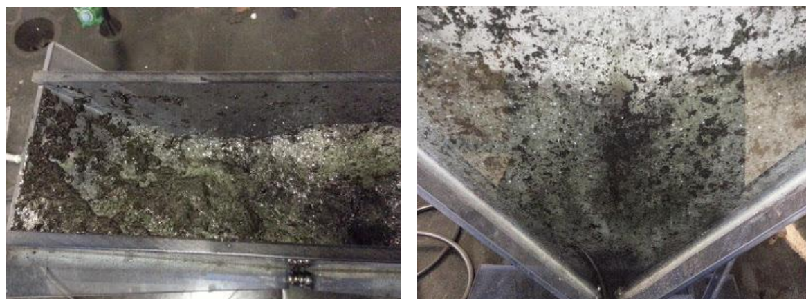
Figure 4.20; Images of froth lifting Nyex™ particles from the adsorption zone of the Arvia Y-cell.
