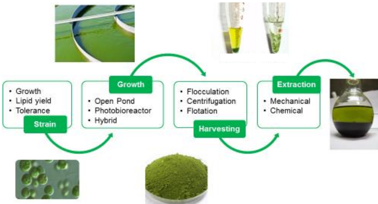
Figure 2.5: Schematic diagram of the stages for lipid recovery from microalgae cells.
