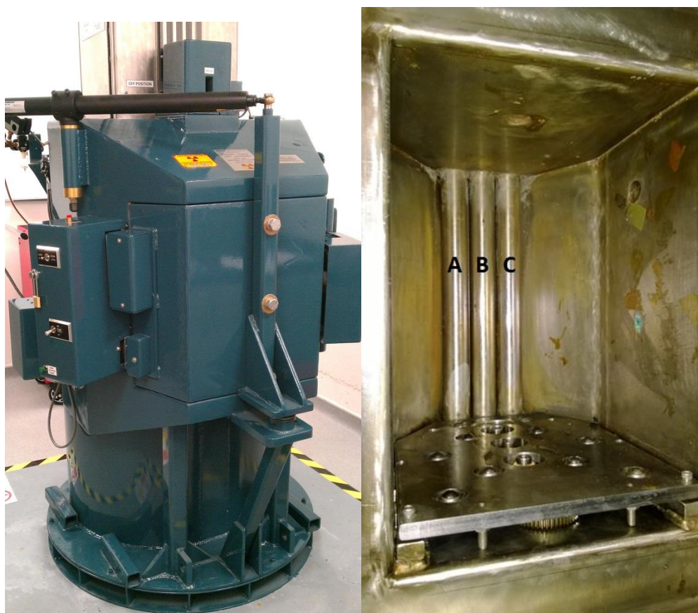
Figure 9: Image on the left shows the Model-812 Irradiator. On the right is the inside of the irradiator showing the three guide rods that contain the cobalt-60 source during irradiation.
