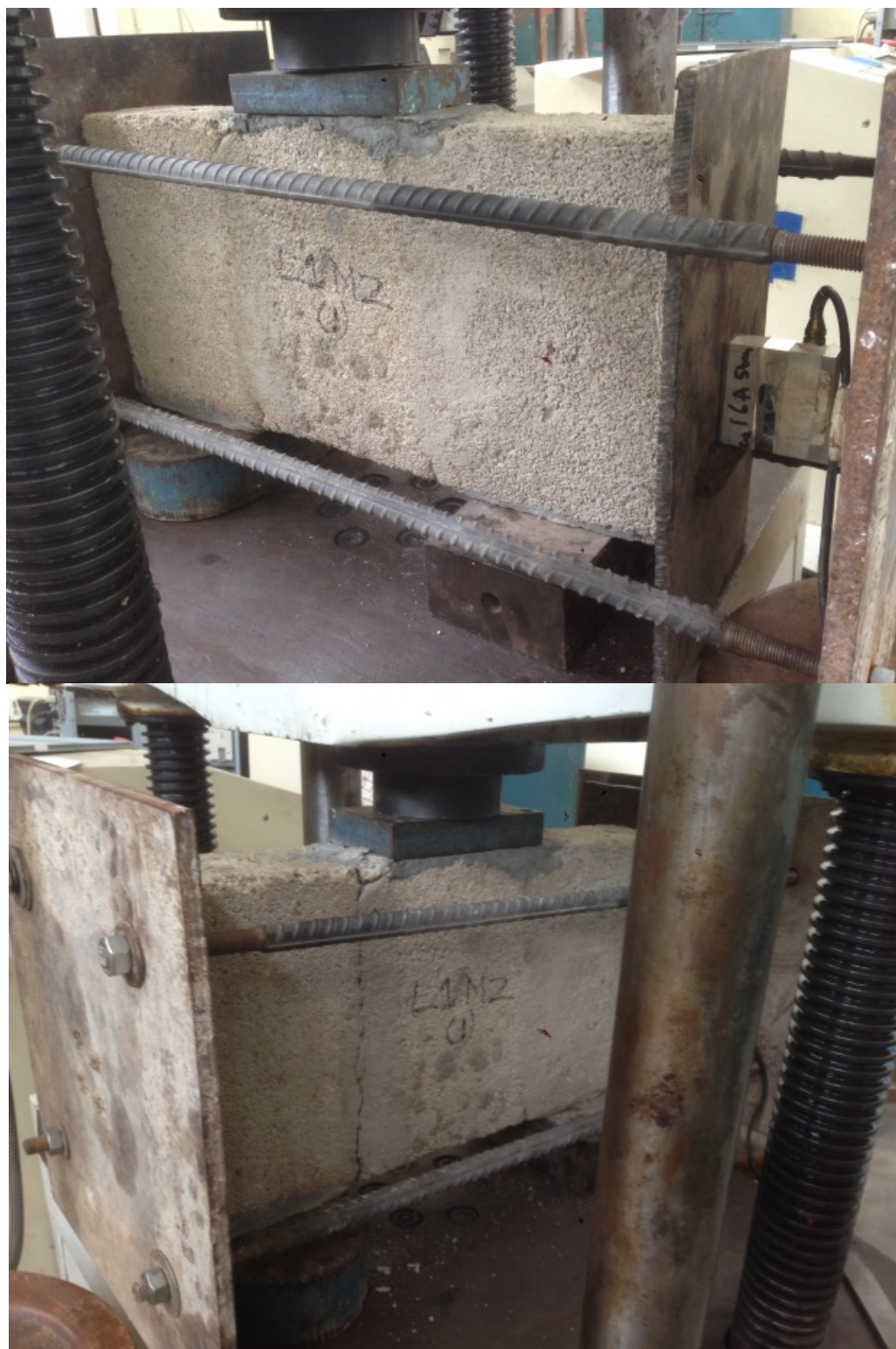
Figure 5.12: Initial shear strength test for concrete blocks
