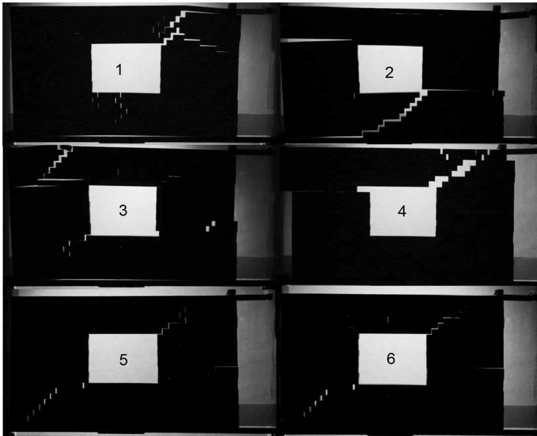
Figure A.9: Glued wall-with-opening specimens at 6 mm base displacement
