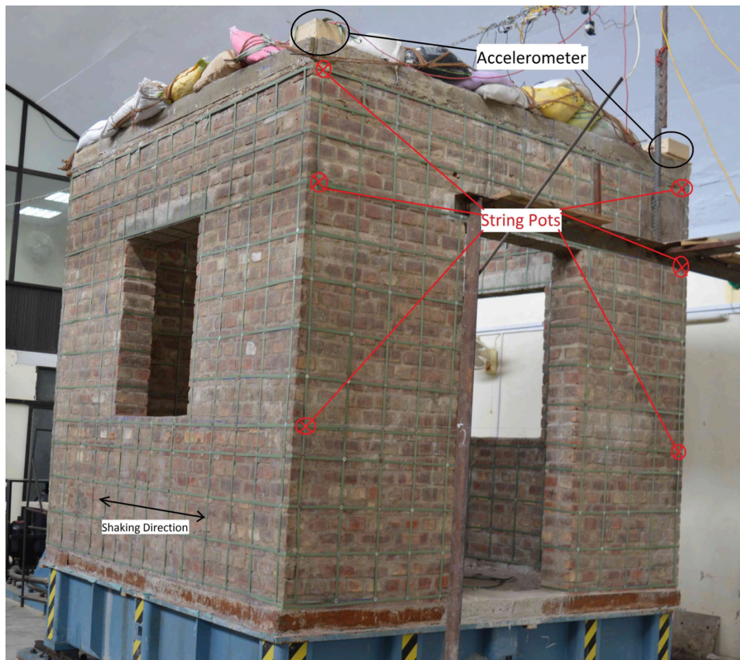
Figure 7.5: Instrumentation for Room-1
