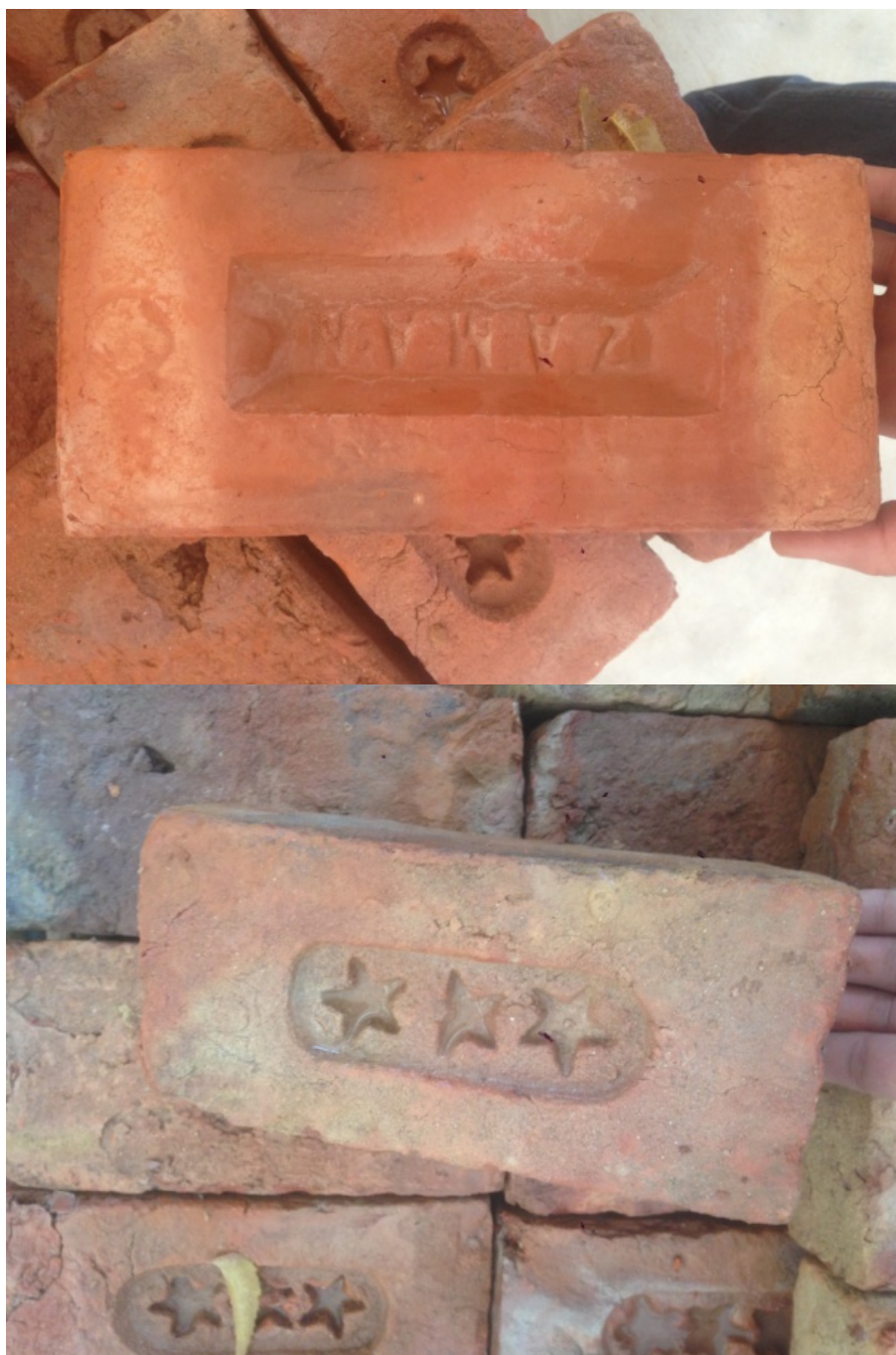
Figure 5.1: Machine pressed brick - R1 (top); Hand pressed brick - R2 (bottom)
