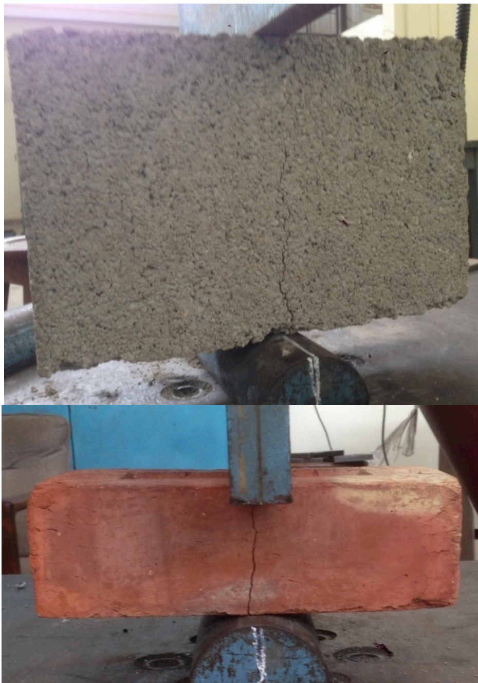
Figure 5.10: Tensile splitting test for concrete block ( top ); red brick ( bottom )
