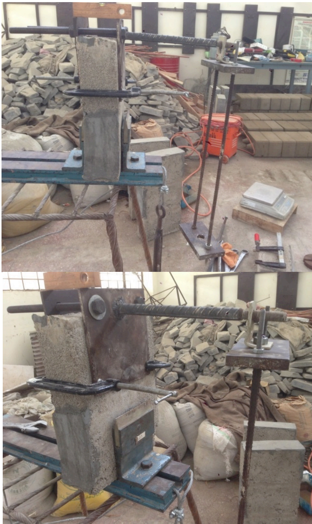
Figure 5.16: Bond Wrench test setup
