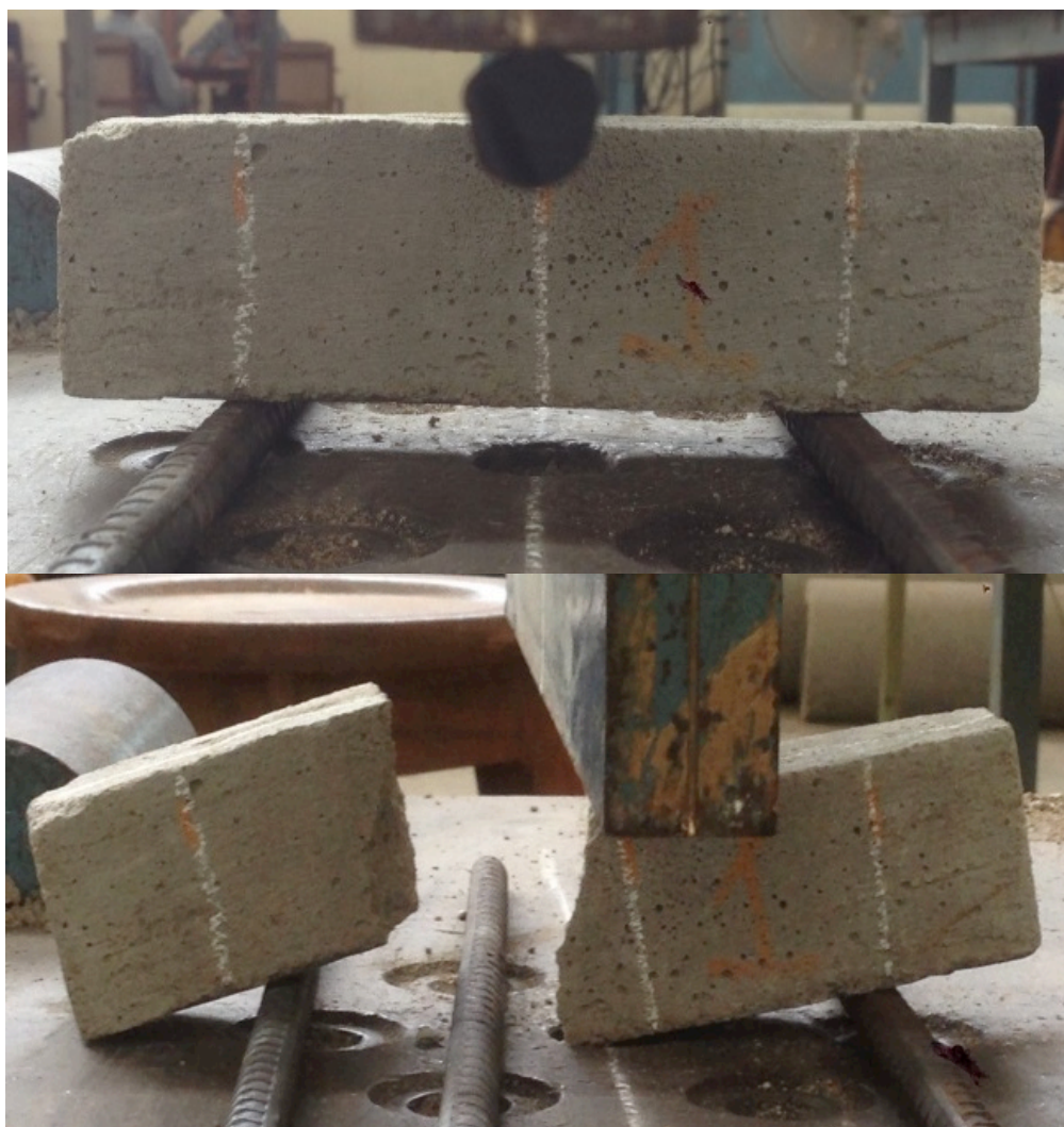
Figure 5.11: 3-Point bending test for mortar
