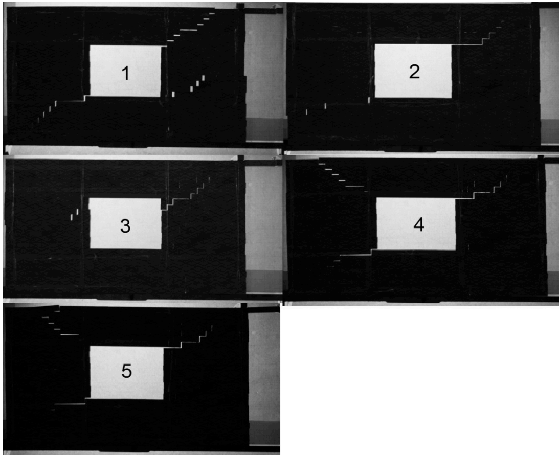
Figure A.10: Retrofitted glued wall-with-opening specimens at 6 mm base displacement
