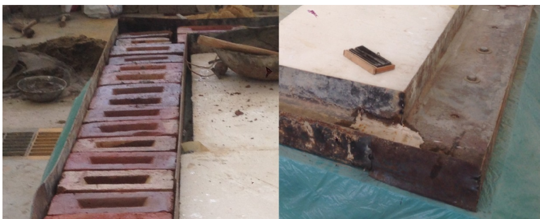
Figure 6.1: Steel channel base used as rigid foundation for masonry wallettes
