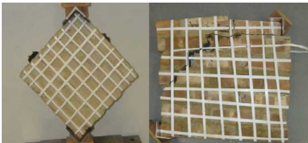
Figure 2.21: PP-Band Mesh Reinforced Specimen Before and After Test [62].
