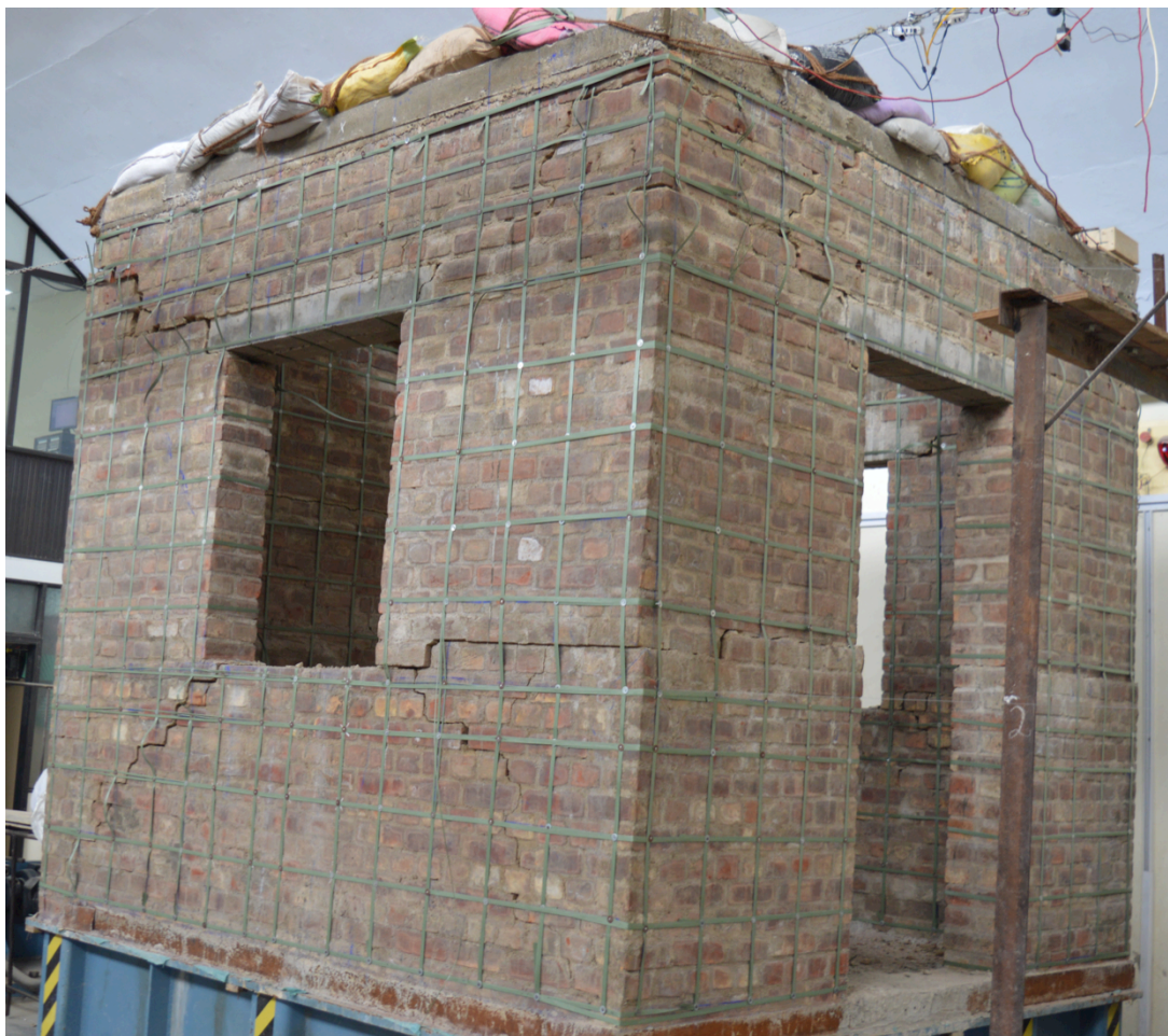
Figure 7.13: Cracks in Room-1 after the initiation of Grade-3 damage in wave-2
