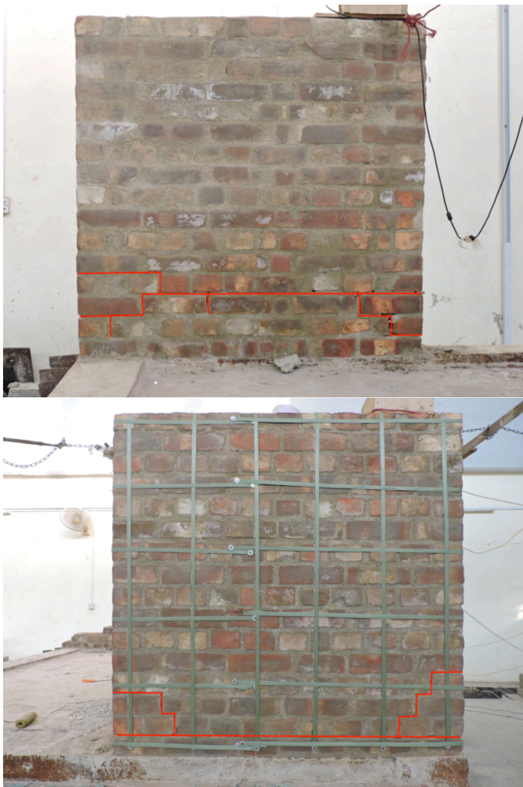
Figure 6.7: Non-retrofit ( top ) and retrofit ( bottom ) specimen at cracking (Grade-3)
