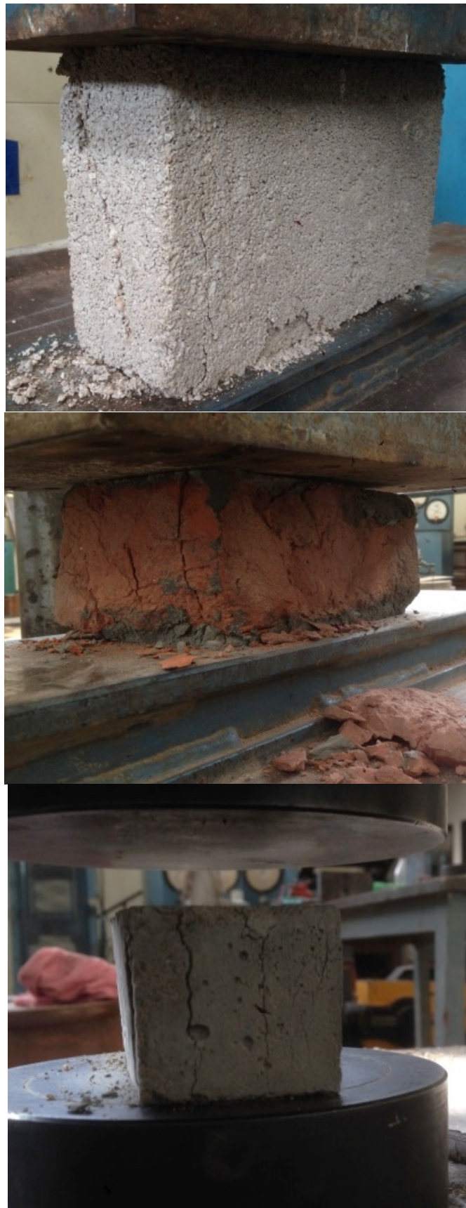
Figure 5.9: Compression Test for Concrete Block ( top ); Red Brick ( centre ); mortar ( bottom )
