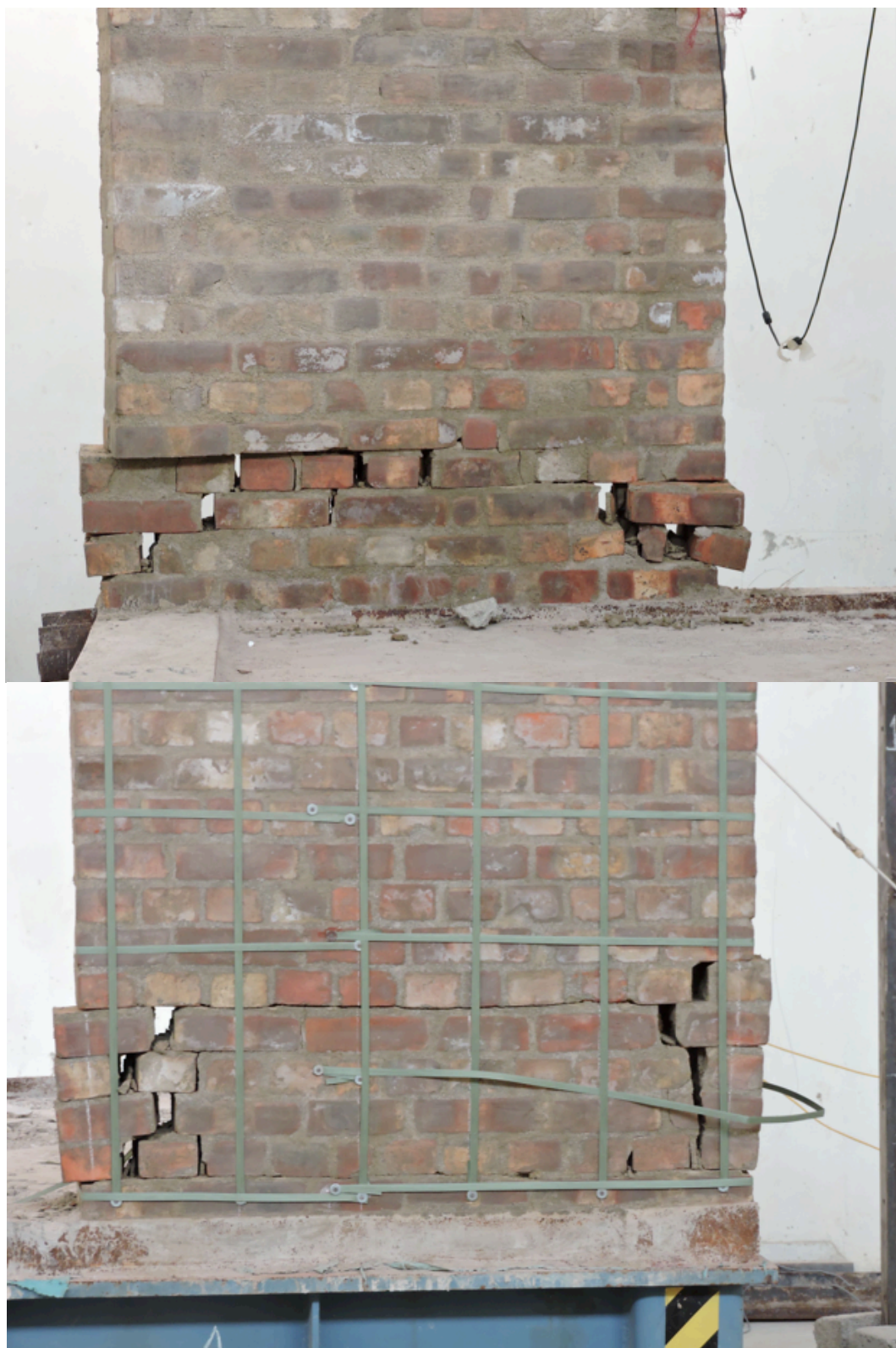
Figure 6.8: Non-retrofit ( top ) and retrofit ( bottom ) specimen before collapse (Grade-4)
