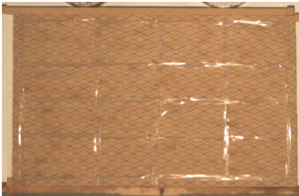
Figure 4.3: Retrofitted solid wall
