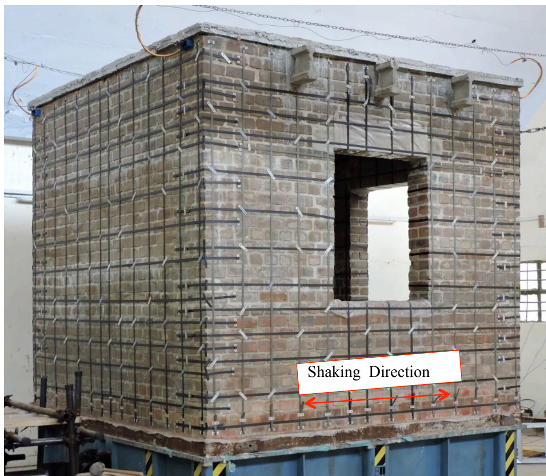
Figure 7.8: Orientation of Room-2 on shake table
