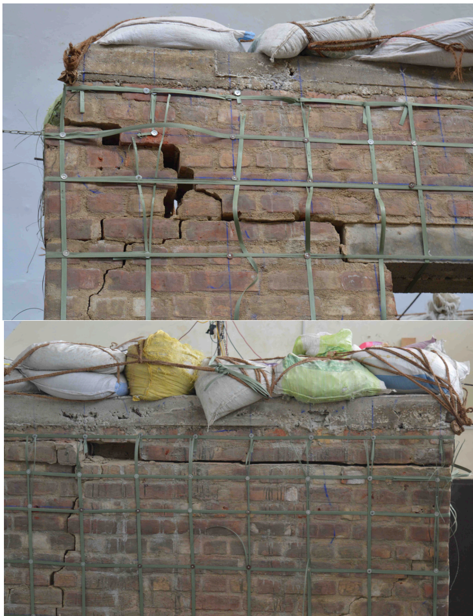
Figure 7.15: Rupture of PP-bands due to the selected connection technique
