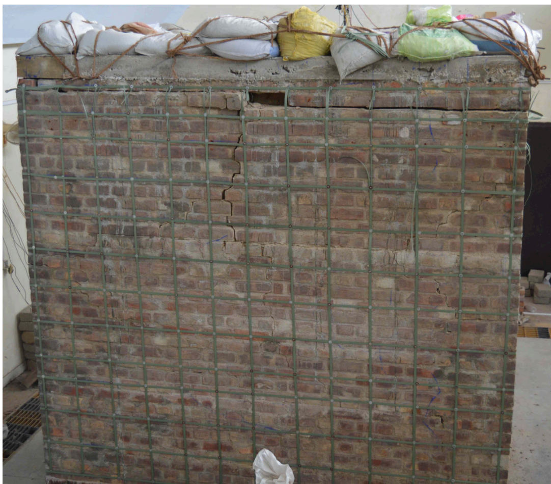
Figure 7.14: Cracks in solid wall of Room-2 at initiation of grade-3 damage
