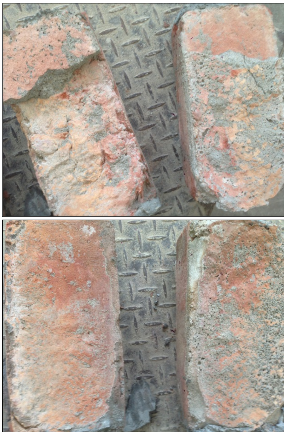
Figure 5.15: R2M1 samples after Initial shear strength test
