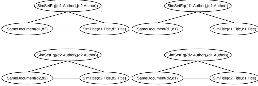
Figure 4.2: The Markov network created by grounding the first rule in Listing 4.1 using two individuals
