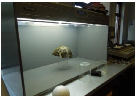
Figure 3.10: VeriVide Light Cabinet used for the front view images.
