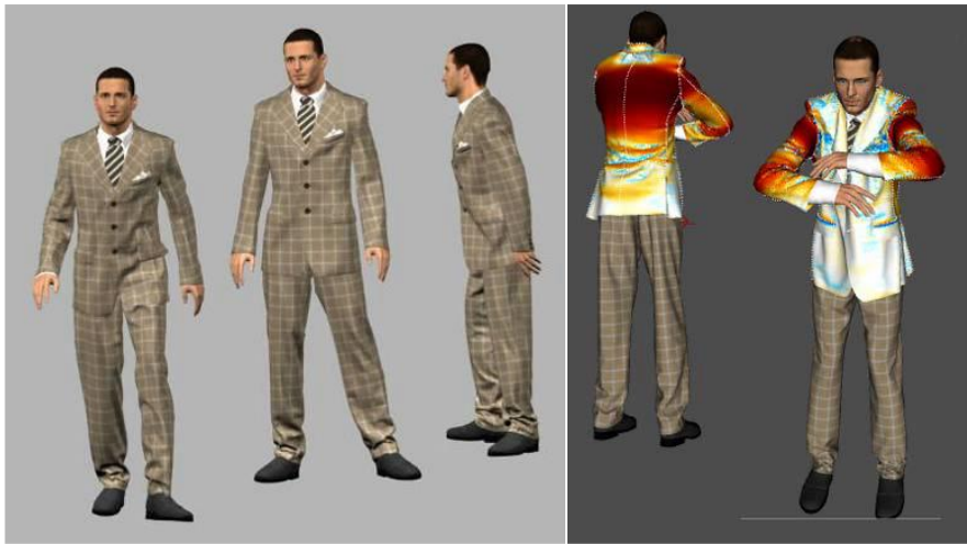
Figure 2.2: Virtual prototyping of men suits visualizing numerical fitting data (Miralab-University of Geneva), source: Luible 2008.
