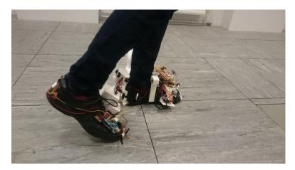
Figure 3.17: Image of the system undergoing validation. Here we can see the left foot is on the ground, signalling that ZUPT and HDR corrections should be applied.
