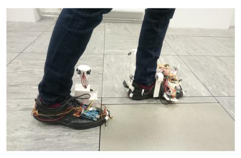
Figure 4.12: Picture showing both feet on the ground during walking. At this point ultrasound measurements are taken giving the displacements between the two feet.
