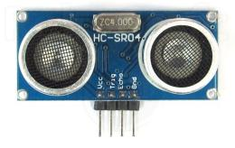
Figure 4.6: The HC-SR04 ultrasound sensor. The transducer to the right is the receiver while that on the left is the transmitter. Additionally, we can see the crystal clock mounted across the top as well as the trigger and echo pins.
