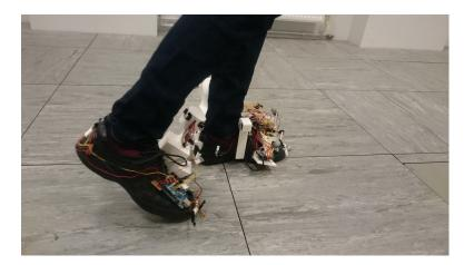
Figure 3.18: Image of the system undergoing validation. Here we can see the left foot is on the ground, signalling that ZUPT and HDR corrections should be applied.
