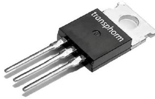
Figure 2.13: GaN cascode device TO-220 through hole packaged, [113]
