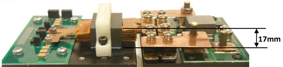
Figure 5.17: Physical implementation of the GaN power converter (side view)
