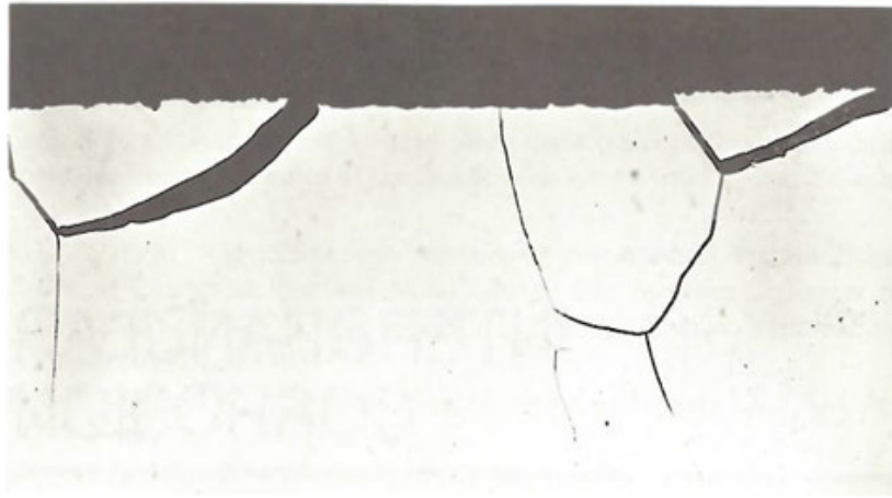
Figure 2.49 Cracks on the grain boundaries caused by sensitization in austenitic alloy generated by the exposure of boiling sulphuric acid-ferritic solution [150].
