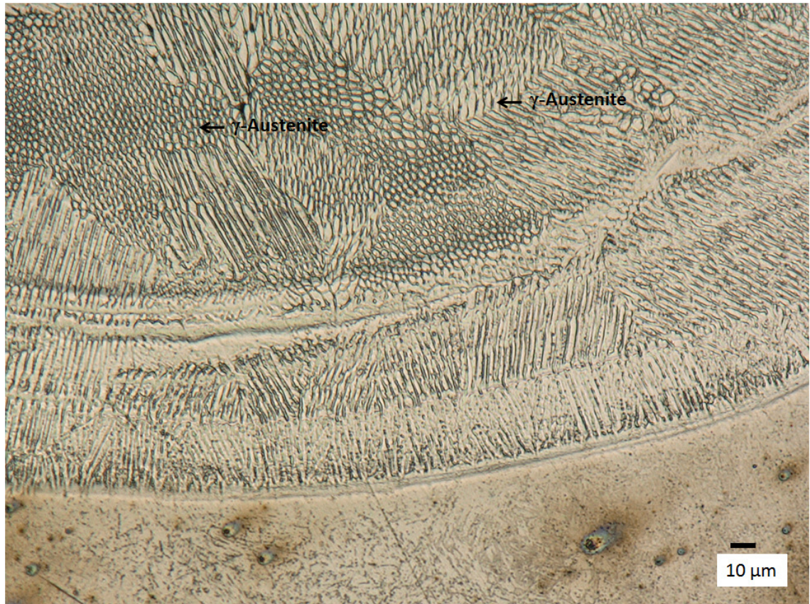
Figure 4.8 Optical micrographs showing the clad layer microstructure developed with a laser power of 850W, a traverse speed of 360 mm.min -1 , and a powder mass flow rate of 4.56 g.min -1 . The appearance of \gamma -austenite phase microstructure is observed in clad bead with no evidence of martensite.
