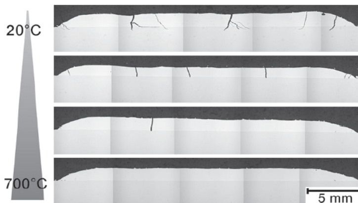
Figure 2.22 Decrease in frequency of cracking with increase in substrate preheating temperature for Stellite 20 coatings deposited on AISI 1045 base material [2].
