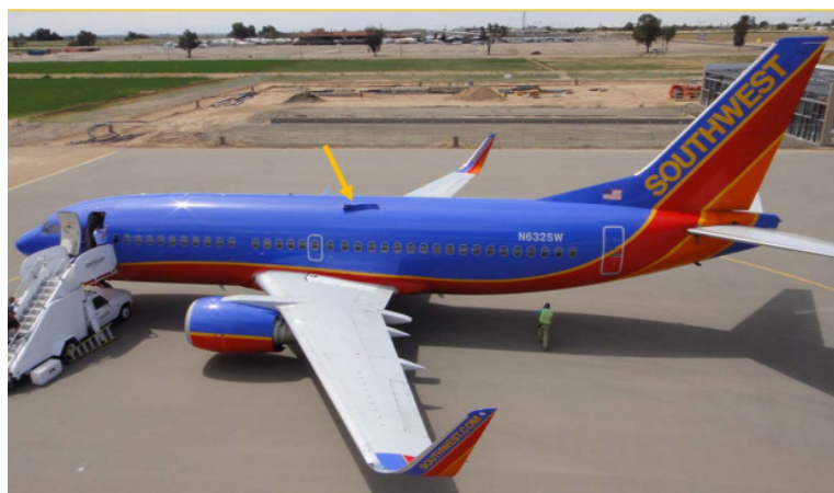
Figure 1.4: Photograph of Southwest airliner with a hole in the upper left fuselage [4]
