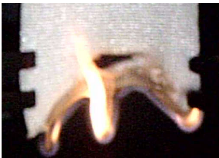
Figure 5.9; PA6 internal flame testing – flaming drips
