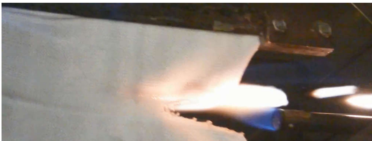
Figure 5.4; DIN 4102-B2; 0.4% FF Exolit 1230 – flaming drips
