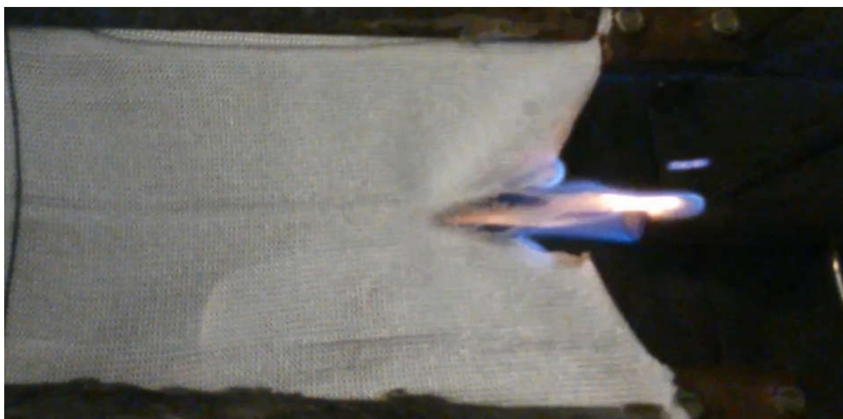
Figure 5.3; DIN 4102-B2; PA6 Control – burning drips.
