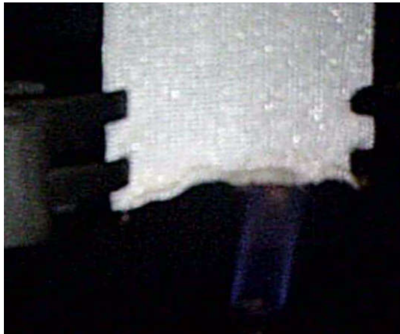
Figure 5.8; PA6 internal flame testing – melting away from flame
