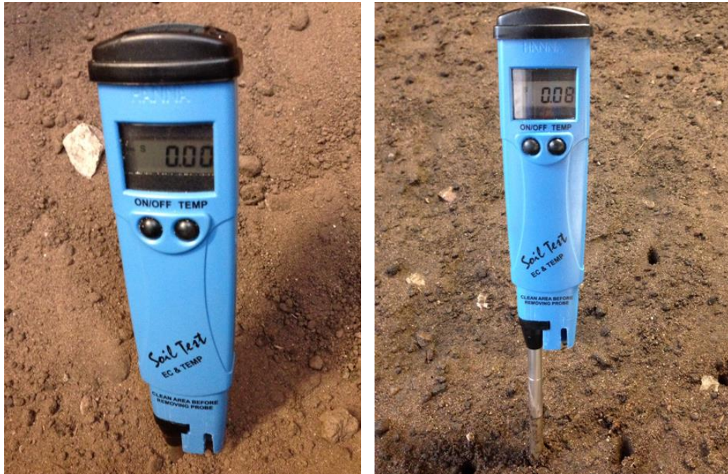
(a) Measured conductivity in the dry soil. (b) Measured conductivity in the wet soil.
