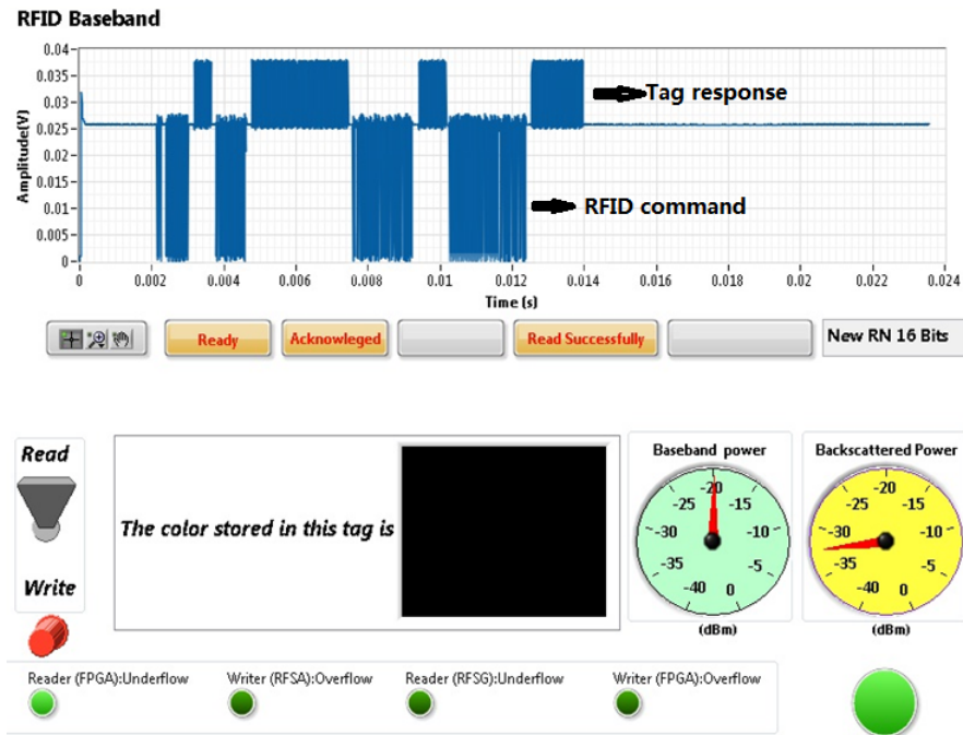
Figure 7.23: The LabVIEW GUI screenshot when implementing the function of reading tag at the operating frequency of 870 MHz and the transmit power (VSG) 9 dBm.
