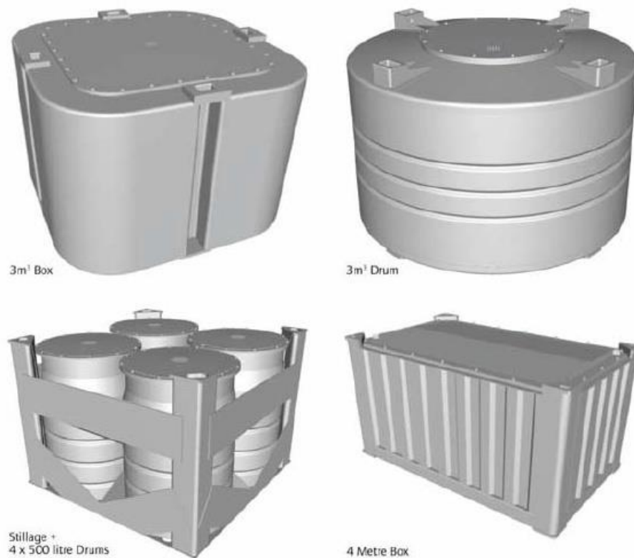
Figure 1-1: Standard waste containers for ILW [6]
