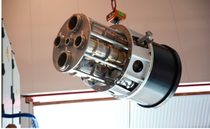
Figure 2.3: The MFI receiver before installation at the observatory. The black cylinder at the back of the MFI is the 20 K cryostat that houses the MFI LNAs. At the front end, the five original MFI receiver feed horns can be seen. The 10 to 20 GHz feeds are the four horns distributed off-centre. The smallest central horn was originally a 30 GHz feed that was removed before commissioning began. Image courtesy of the QUIJOTE Collaboration.
