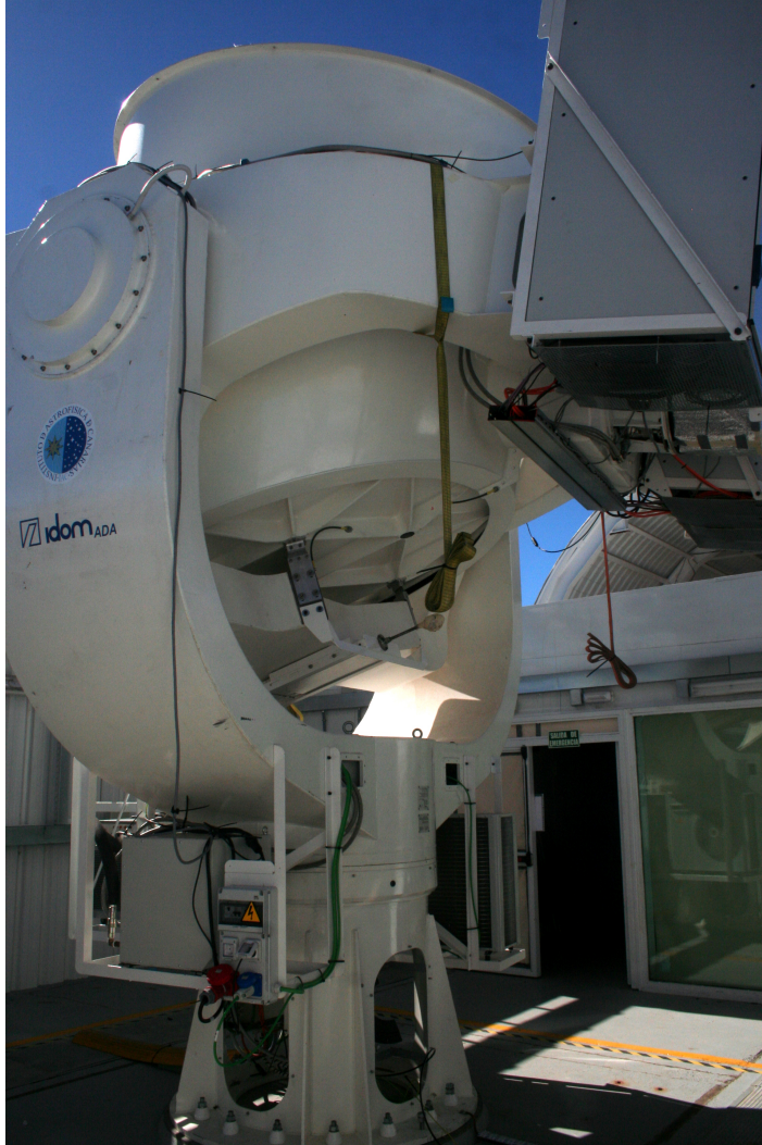
Figure 2.2: QUIJOTE QT1 alt-azimuth mounted telescope inside the dome at the Izaña observatory pointing towards the zenith position. The MFI receiver BEM is stored in the cabinets on the right side of QT1. Between the BEM cabinets is the MFI FEM and cryostat.
