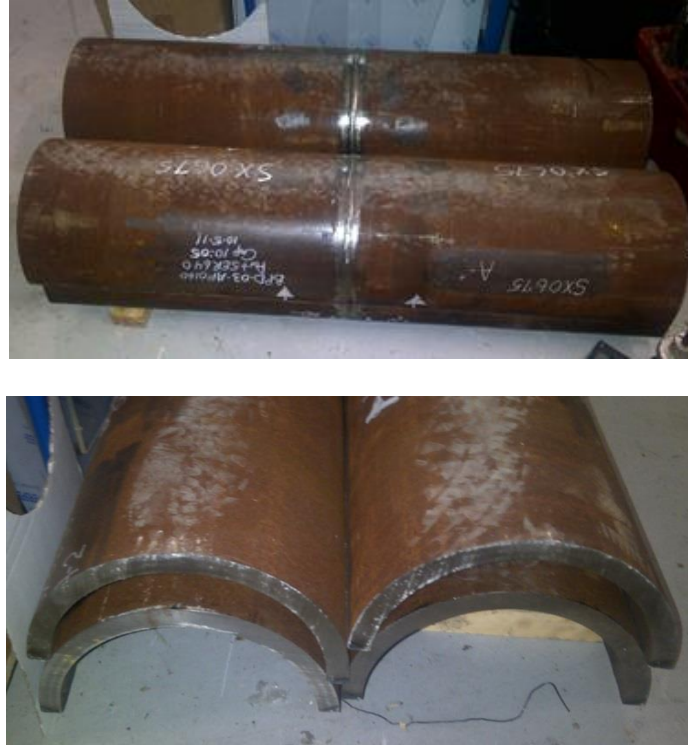
Figure 3.2 As-received sections of the linepipe from which test samples were manufactured.
