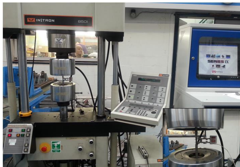
Figure 3.12 Experimental set-up for cyclic strain-controlled fatigue testing. Inset: configuration showing grips, specimen and extensometer.
