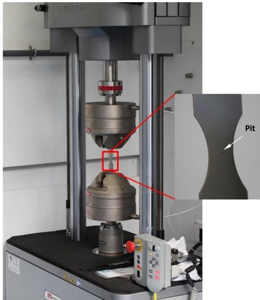
Figure 3.14 Experimental set-up for in-air fatigue testing. Inset: gauge section of fatigue specimen containing a corrosion pit.
