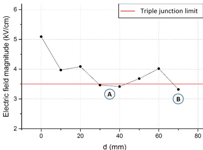
Fig. 6. Maximum electric field magnitude at the triple junction against the distance ( $d$ ) of the grounded-end grading device from the edge of the compression insulator end-fitting. At positions A (30 mm - 40 mm) and B (70 mm) the electric field magnitude is reduced below the 3.5 kV/cm limit.
