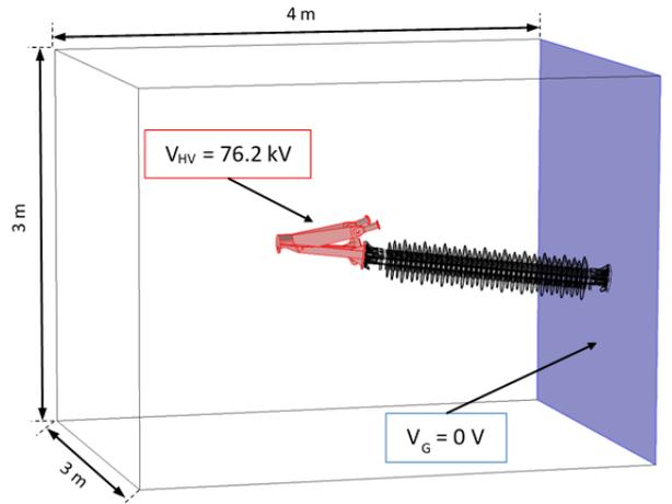
Fig. 2. Computation domain with 132 kV ICA model. The right-most surface of the domain is grounded to represent the tower which is omitted to simplify the calculation.
