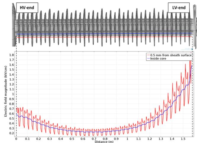
Fig. 10. Electric field magnitude on the surface and inside the core of the compression insulator at 132 kV.
