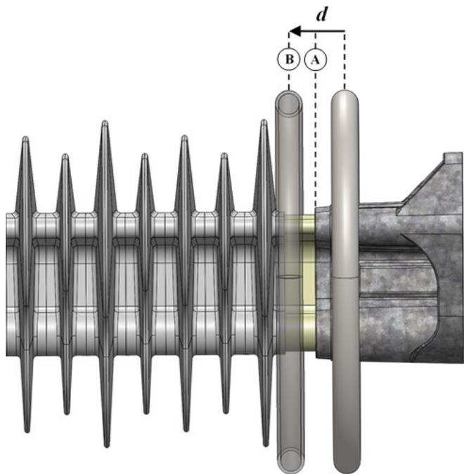
Fig. 5. Grounded end grading device position variation (parameter  $d$ ) and optimal positions A and B.
