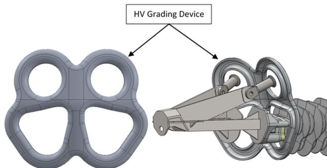
Fig. 8. HV grading device for the 132 kV ICA
