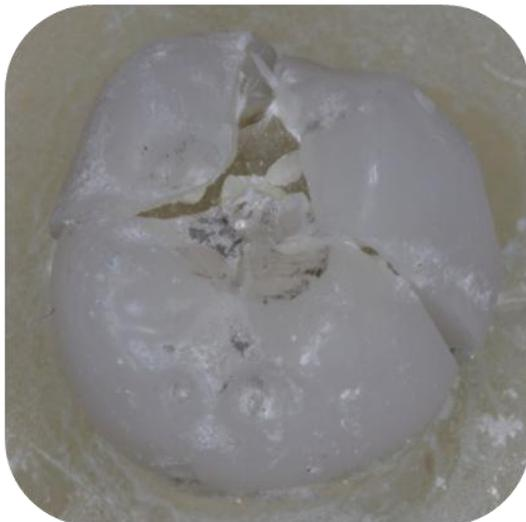
**Figure 9.6:** Fractured representative specimens from each group. Lava Zirconia: LZ (top) Lava Ultimate: LU (mid), FRC-S (bottom)
