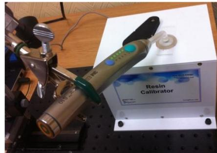
**Figure 3.4:** MARC resin calibrator used for irradiance measurement, A) its main parts, B) LED curing unit during the baseline measurement and C) the mould assembly placed on top sensor prior to irradiance measurement.
