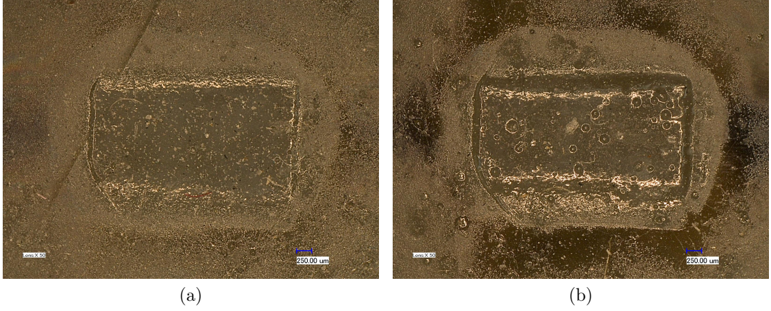
Figure 4.13: Optical images of square crater produced by excimer laser on epoxy using 1.5 \text{ J/cm}^2 laser fluence, (a)100 NOP and (b)200 NOP.
