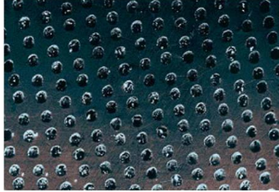
Figure 2.38: Laser Surface texturing of regular micro-surface structure in the form of micro-dimples with diameter of 100\ \mu\text{m} , depth of 10\ \mu\text{m} and dimple density of 20 % [161].
