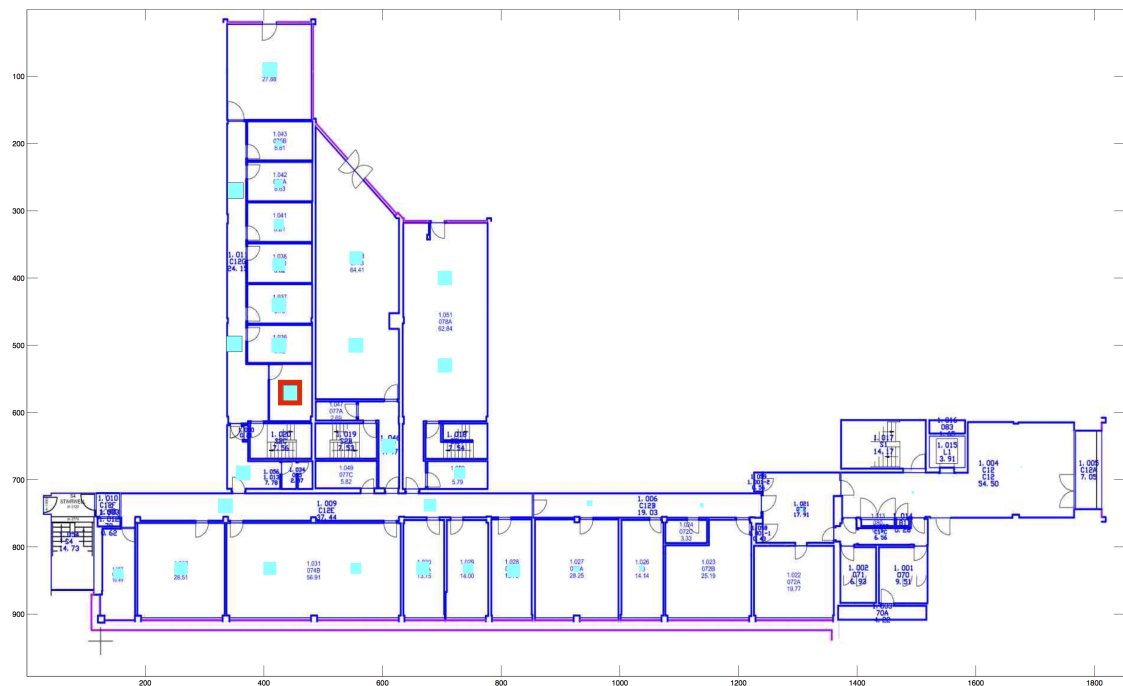
Figure 6.21: Position display based on WAPs presence. The pale blue squares indicate the rooms containing at least one matching WAP. The larger the size of the square, the larger the number of matching WAPs. The room with the largest number of matching WAPs is marked with a red edged square.
