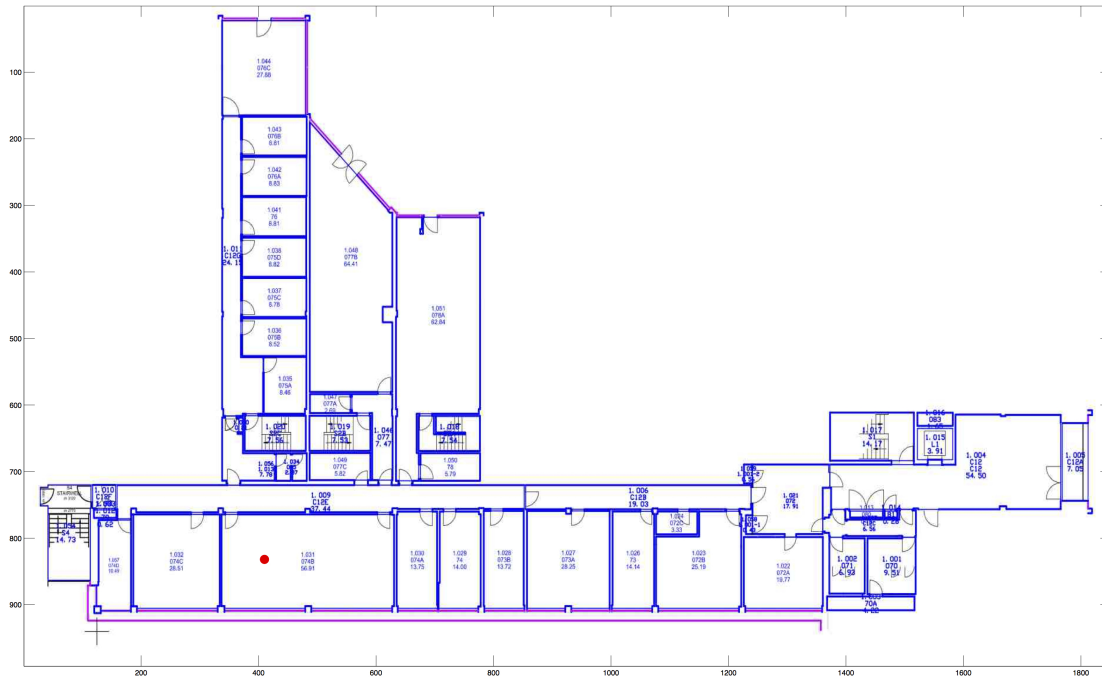
Figure 6.22: Position display based on WAPs RSSI. The room with the smallest RMSE is marked with a red dot on the floor plan.
