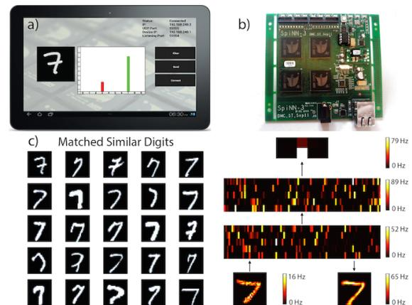
Fig. 1. Handwritten digit recognition setup. a) The user interface running on a mobile device, showing a finger-drawn digit (left) and a correct classification. b) A 4-chip SpiNNaker board. c) The output of the laptop monitor, showing network-classified similar digits from the training set, as well as the firing rates of neurons within each layer during classification
