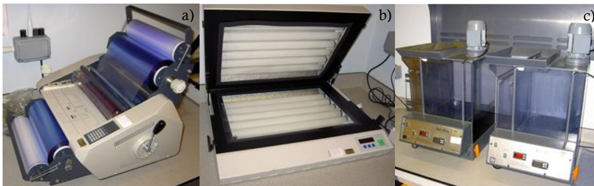
Figure 6.7: Apparatus used for photochemical milling of iron foil: a) GX 12 inch dry laminator; b) Mega-electronics y80 Ultraviolet light box; and c) 2 fine-line rotary etch solution developing units
