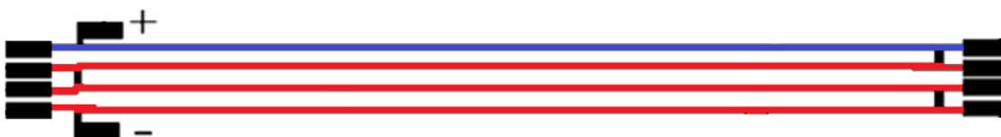
Figure 6.1: Initial design of ERCM, taken from [1,2]. Suggested sensor use illustrated; corroding filaments in red, reference in blue and the black areas non-monitored conducting pads.
