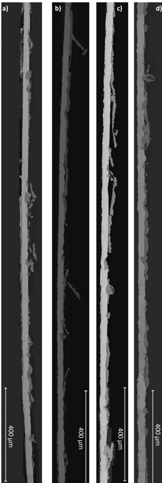
Figure 7.21: Combined Scanning electron micrographs of iron foil cross section after application of pre-corrosion methodology. Corroded surfaces are shown on the right. Foils shown were pre-corroded for;
