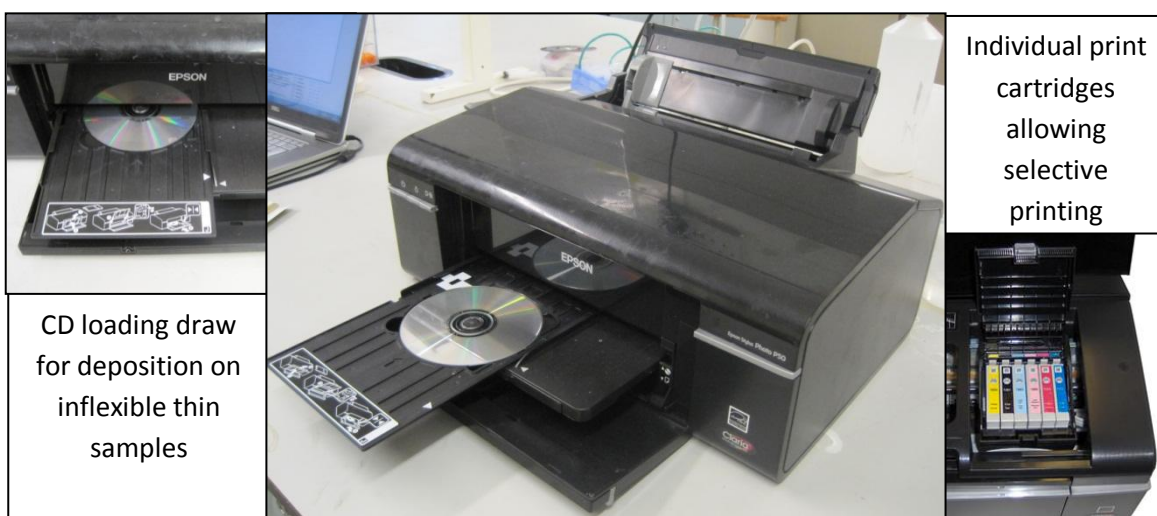
Figure 6.10: Epson Stylus P50 printer used for deposition of sodium chloride
