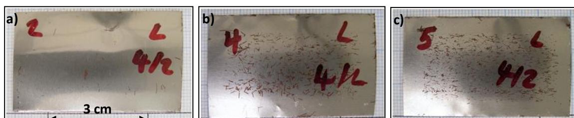
Figure 7.19: Reverse, lacquered side of iron foils, corroded in alternating conditions for 4 repetitions, contaminated by repeat inkjet contamination with NaCl: a) 2 printings; b) 4 printings; and c) 5 printings
