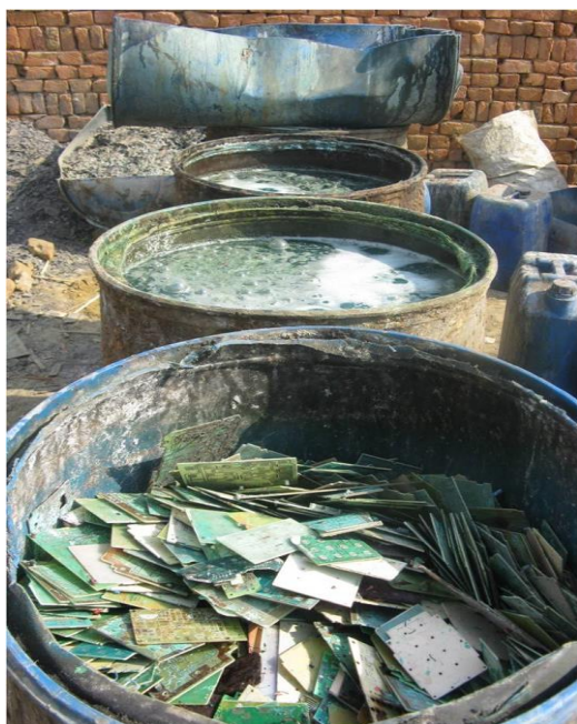
PCBs in Acid bath and Cleaning PCBs in Caustic Soda Solution in Mandoli, Delhi, 2012:
