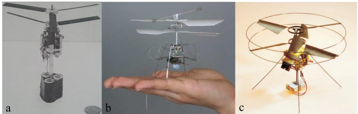
Figure 2.2 Coaxial rotary MAV designs. (a) The University of Maryland ‘MICOR’; image taken from [13]. (b) Seiko Epson ‘ \mu FR-II’; image taken from [14]. (c) ETH Zurich ‘Coax’; image taken from [16].
