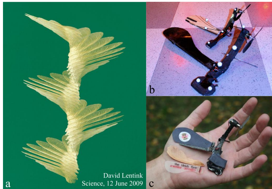
Figure 2.6 (a) The flight path of a maple seed visualized in a composite multiframe photograph; cover photo of Science , June 2009. Winged seed rotating MAV designs: (b) The University of Maryland Samara I and II; image taken from [26]. (c) The University of Maryland Samara III; image taken from [25].
