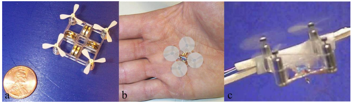
Figure 2.4 ‘Mesicopter’ quad-copter rotary NAV design developed at Stanford University. (a) and (b) Initial prototypes. (c) Four rotor lift test. All images taken from [19].
