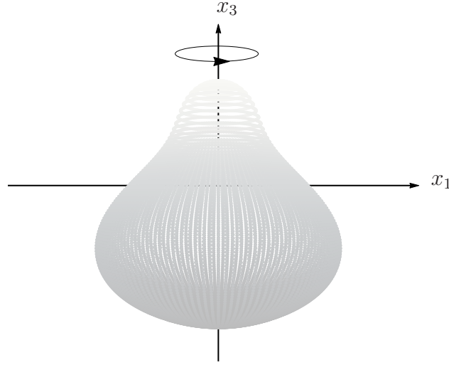
Figure 5.1: An example of a three-dimensional scatterer that is axisymmetric about the x_3 axis.
