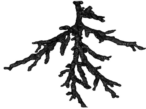
Figure 4. The imported XCT geometry for modelling in FEA. The tree is 59\ \mu\text{m} long.
