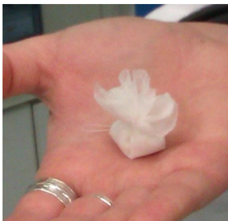
Figure 2.39: Immobilised TIL wrapped in first aid gauze ('tea bag') as set-up for recycling experiments
