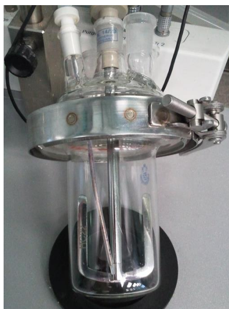
Figure 2.37: EasyMax TM reaction vessel with stirring anchor and temperature probe
