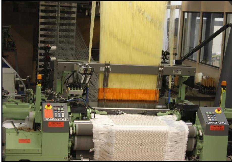
Figure 3.1 Rapier weaving machine equipped with Jacquard
