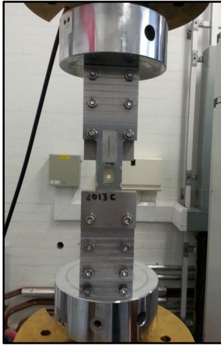
Figure 6.3 Test fixtures for open hole compression test
