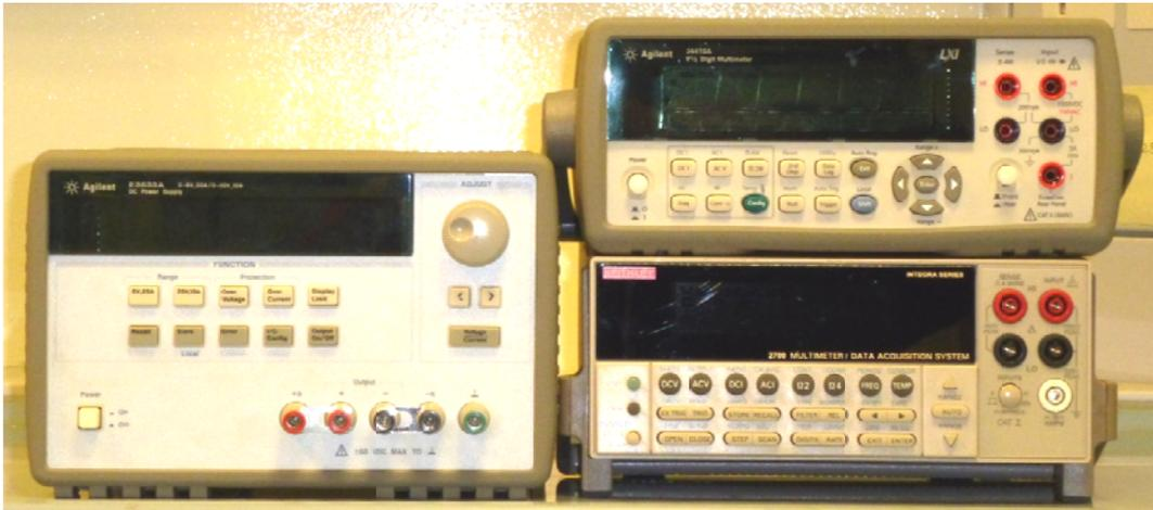
**Figure 63: Photograph of digital multi meters and Agilent DC power supply**
