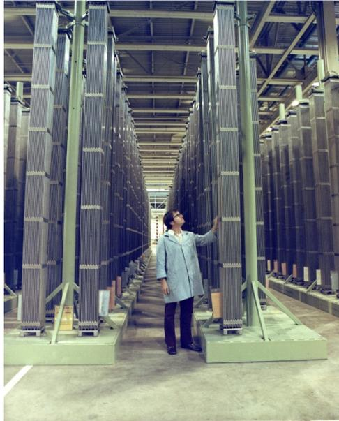
**Figure 112. Westinghouse PWR fuel assembly. (ORNL Photo 3897-77)**
