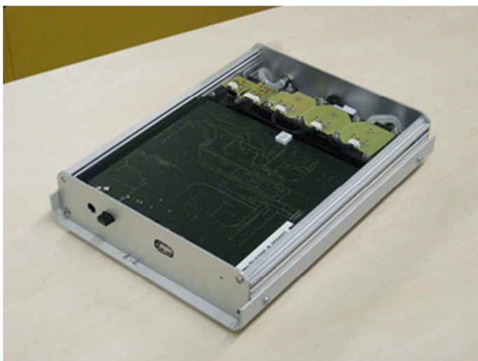
Figure 188 Air monitoring sensor unit open top and front view.
