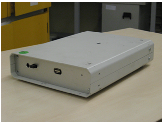
Figure 186 Air monitoring sensor unit front view.
