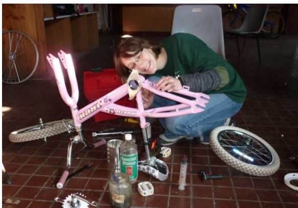
Figure 4-3: Cleaning the bottom bracket of a children's bike at a Recicleta repair day. 11/06/2011. Photo courtesy of Felipe Cuevas.
