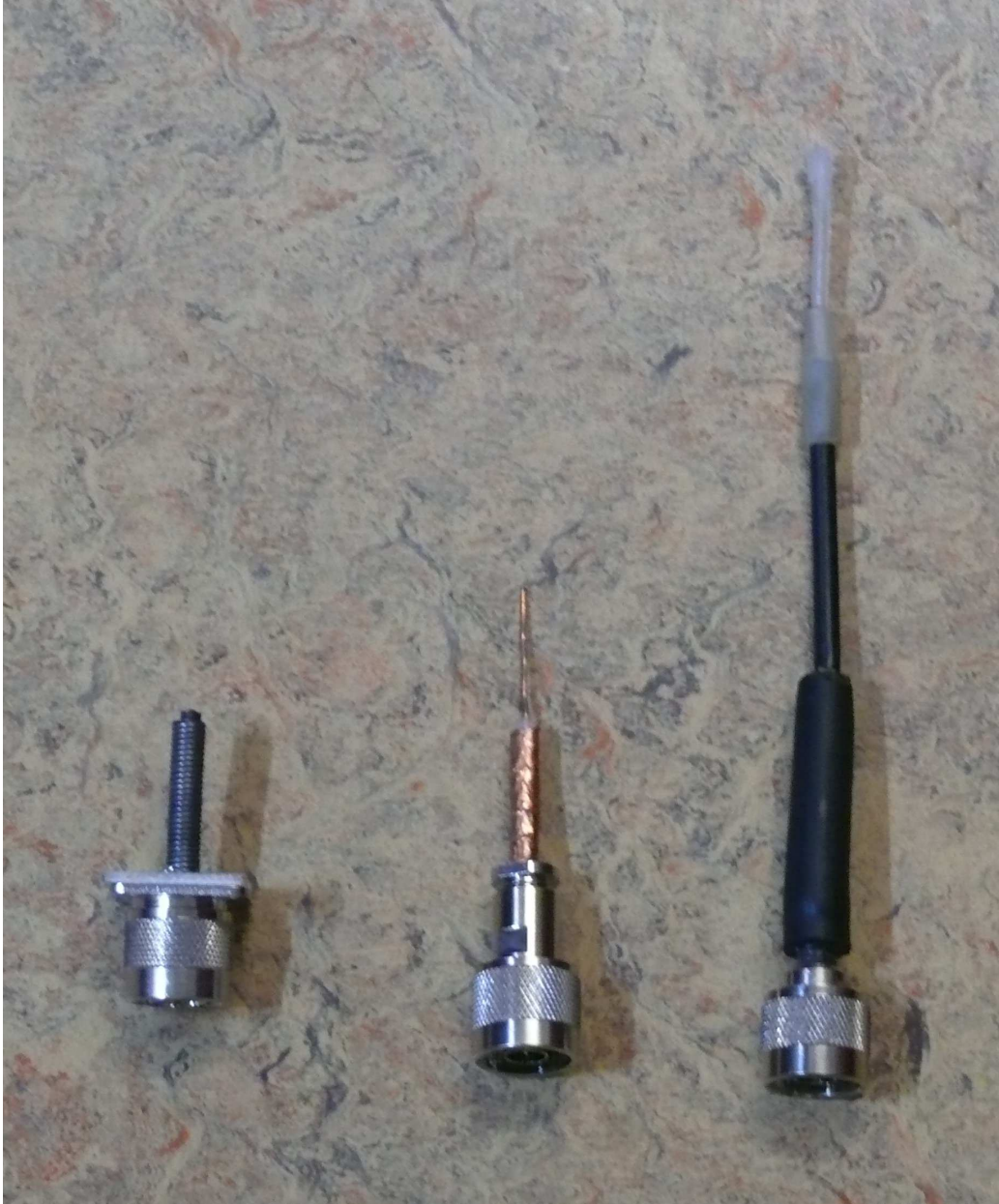
Figure 4.14: Antennas used during field work. Left: “Sprung monopole”, Centre: “improvised coax monopole”, Right: “final coax monopole”.
