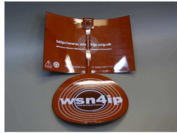
Figure 7. Flexible ring monopole antenna with conformal flexible ground plane
