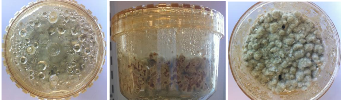
FIGURE 2.15: Water formation in the bioreactor system (a) on the lid, (b) on the wall and (c) inside the bioreactor. Pictures are from the current study
