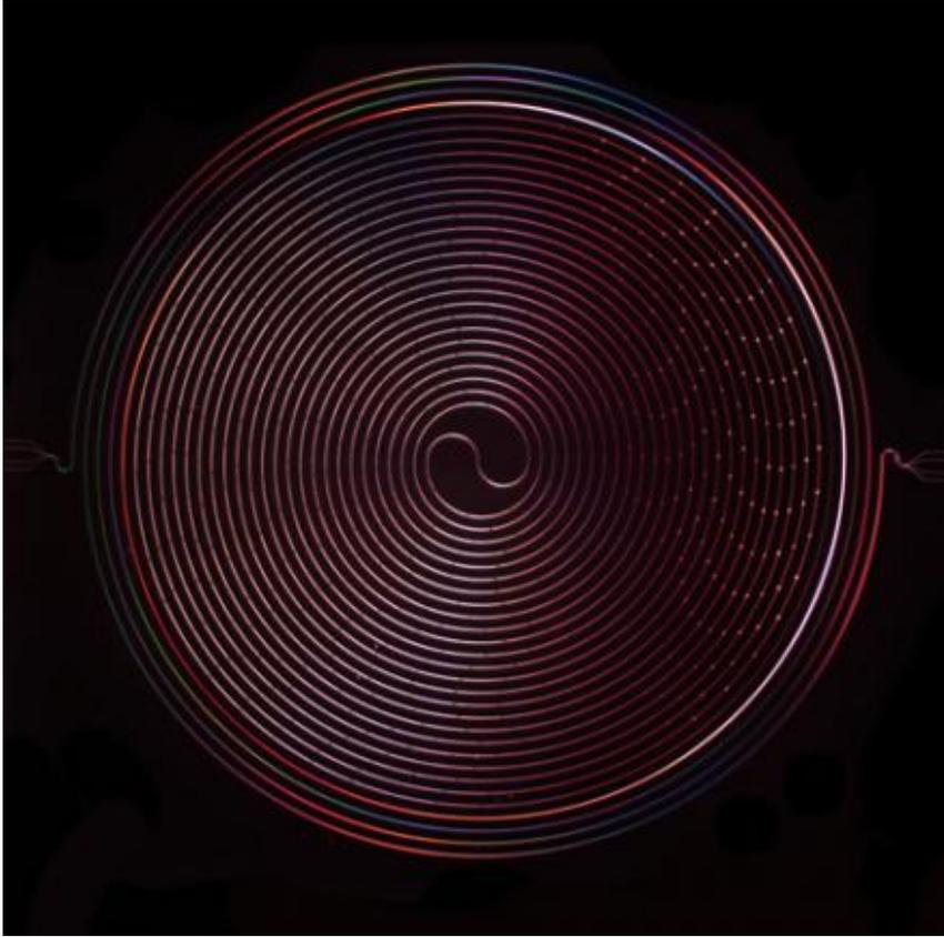
Figure 6.2.3: 0.8 m long travelling wave superconducting parametric amplifier. From A New Kind of Amplifier [156].
