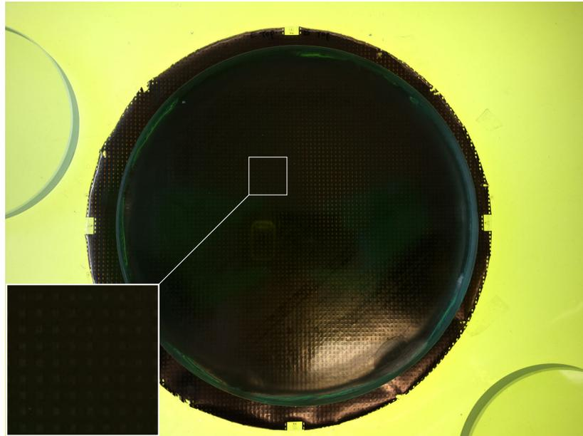
Figure 3.9: Two grids layered on top of one another and held down with a cylindrical glass block. This photo demonstrates a worst case scenario of bad alignment when no light is able to pass through.
