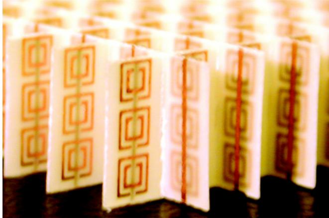
Figure 1.8: A close up the split ring resonator and wire structure used in Shelby et al. (2001b) to demonstrate negative refractive indices. The SRR and wires were printed on opposite sides of the same substrate and together were capable of creating a negative index band for radiation with its  $E$ -field aligned with the wires. To provide a sense of scale the size of the SRRs is 5 mm. Photo taken from Shelby et al. (2001b, figure 1). Reprinted with permission from AAAS.
