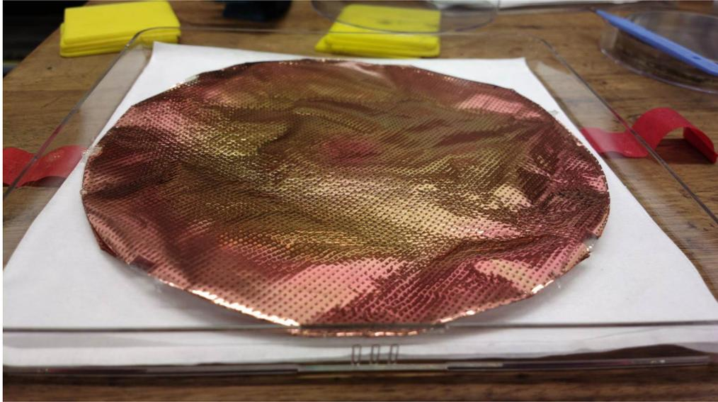
Figure 4.33: Layer A side of the spot welded layers ABCDEF.
