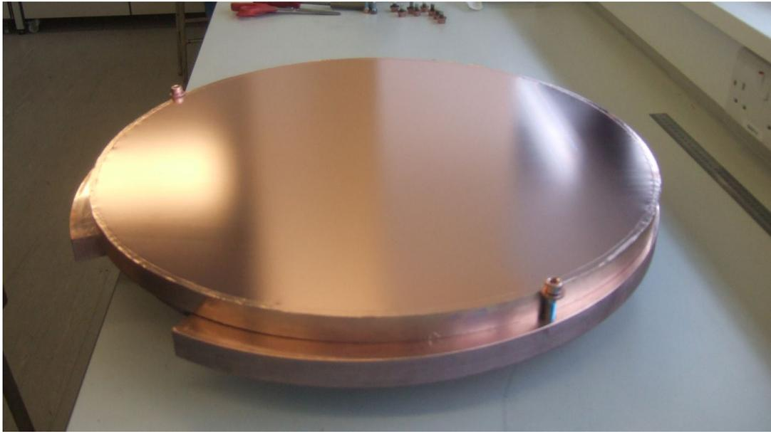
Figure 3.3: A freshly copper coated polypropylene sample 53 cm in diameter.
