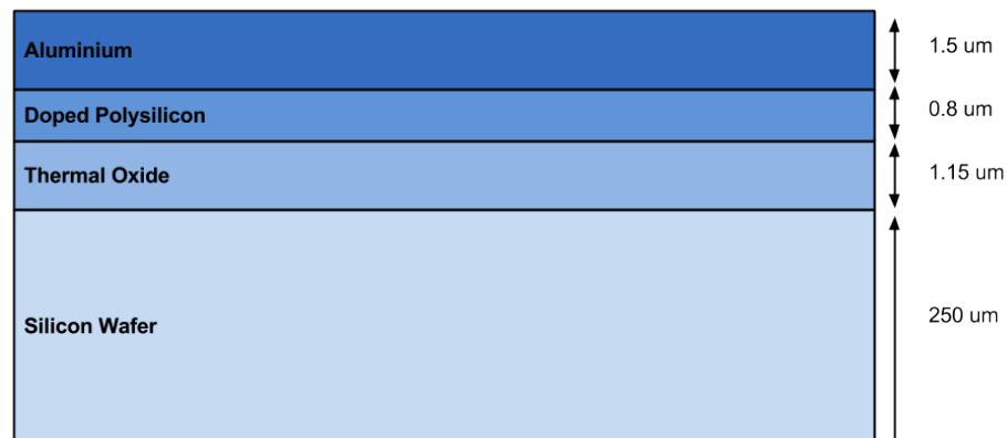
Figure 8.8: Sketch of the layout of the layers on the backside of the simulated 3D silicon detector [97] (not to scale). Antiproton direction is from the top, downwards.
