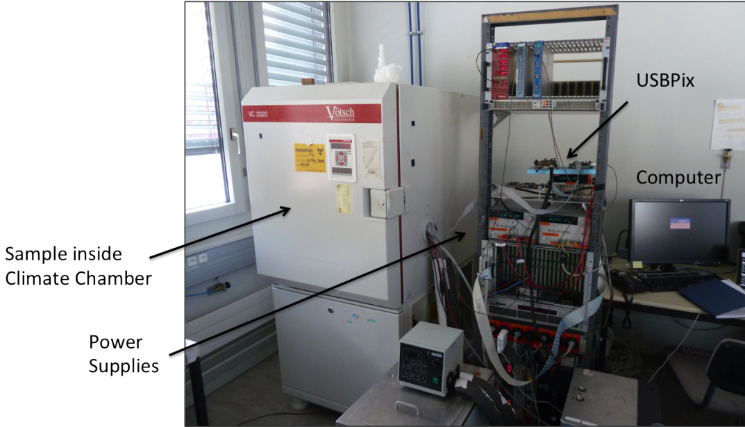
Figure 6.1: Photograph of the laboratory setup at CERN. The USBPix system, the climate chamber, the computer and the power supplies are all labelled as shown.
