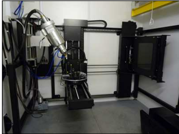
Figure A.1. Nikon Metrology 225/320 kV system.
