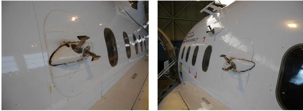
(a) View of modified Rosemount 102E housing from the front looking towards the rear of the aircraft. (b) View of modified Rosemount 102E housing from the rear looking towards the nose of the BAE-146.
