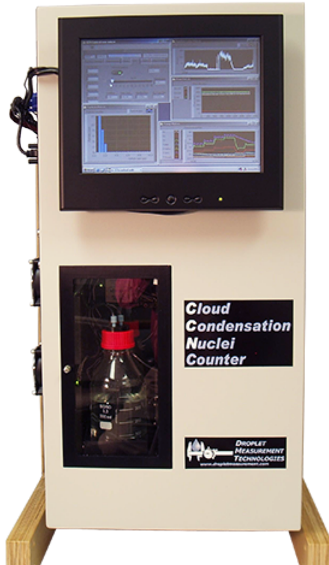
Figure 2.1: Picture of a single column CCNc, courtesy of DMT Inc. Boulder, Co. The dual column CCNc used in this work has the same footprint as this instrument. The deionised water and waste water reservoirs can be seen through the viewing window. The lab view software that controls and stores the CCN data can be seen running on the front mounted touch screen.
