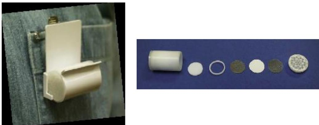
**Figure 8: An Ogawa personal air sampler<sup>51</sup>**
