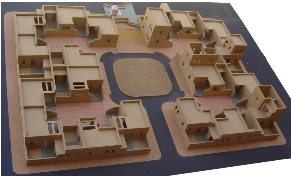
Fig. 4.16: Model of housing cluster at Sadar Nagar. The ‘scale of engagement’ common to traditional Kutchi housing is apparent, (main street; community chowk ; cluster chowk ; domestic falia ; otla ; living room; bedroom), theoretically enabling traditional use. The abstraction of the plan becomes intelligible in a model and was a principal tool of Hunnarshālā in explaining their ideas to the community. Likewise, the intentionally vernacular design of the houses becomes clear. (Photograph by Hunnarshālā, 22.02.2004, adapted by author)
