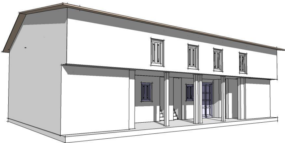
Fig. 4.56: Perspective showing traditional Kutchi 'semi-detached' house with shallow pitched roof and shared verandah. It can be presumed that such a building would house elements of an extended family and would be part of a wider complex of more buildings within a homestead boundary. (Adapted from: ibid. )
