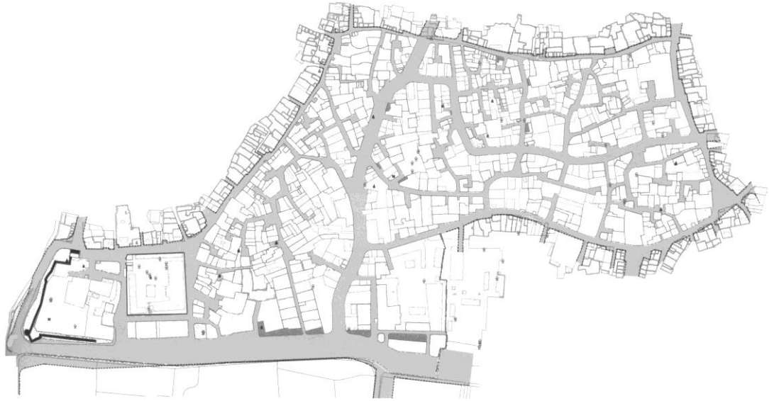
Fig. 4.6: Old Bhuj, post-2001 Development Plan renewal, showing the ‘clarified’ road layout with emphasis placed on porosity and the contingent decline of the pols-like urban form. (Adapted from Tyabji 2006: 238)
