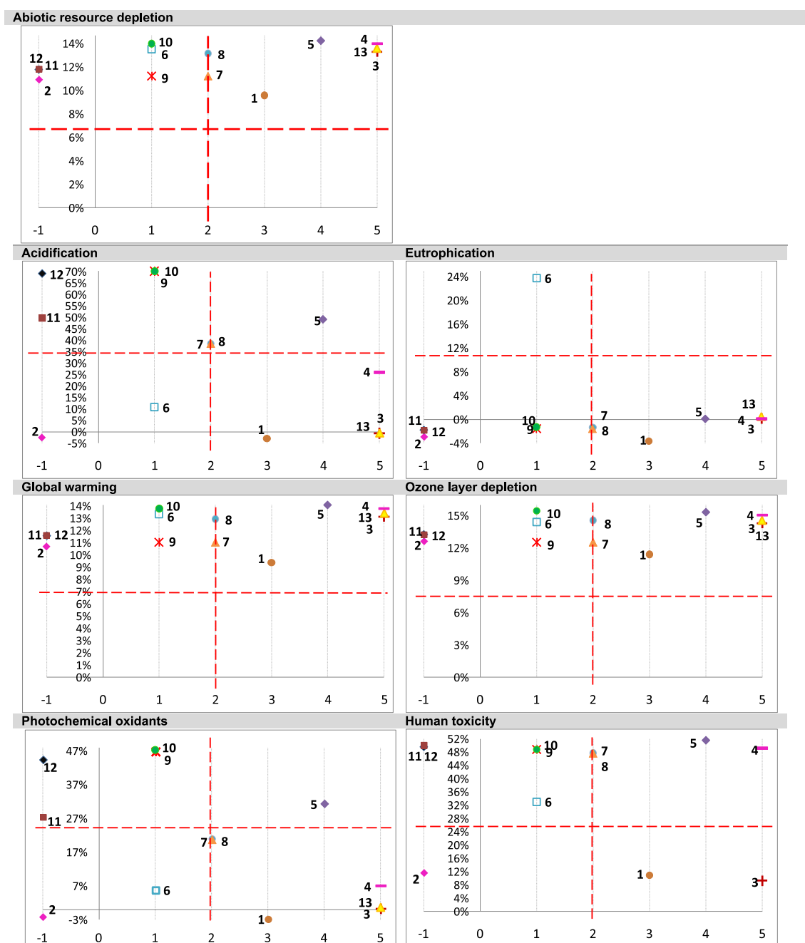
Fig. 9. Eco-efficiency analysis: environmental impact reduction potential (%) vs net annual savings (score). [The broken lines dividing the graphs into four squares represent the eco-efficiency lines as defined in Fig. 2 and Section 2.4.1. The options in the top right-hand corner are considered eco-efficient.].
