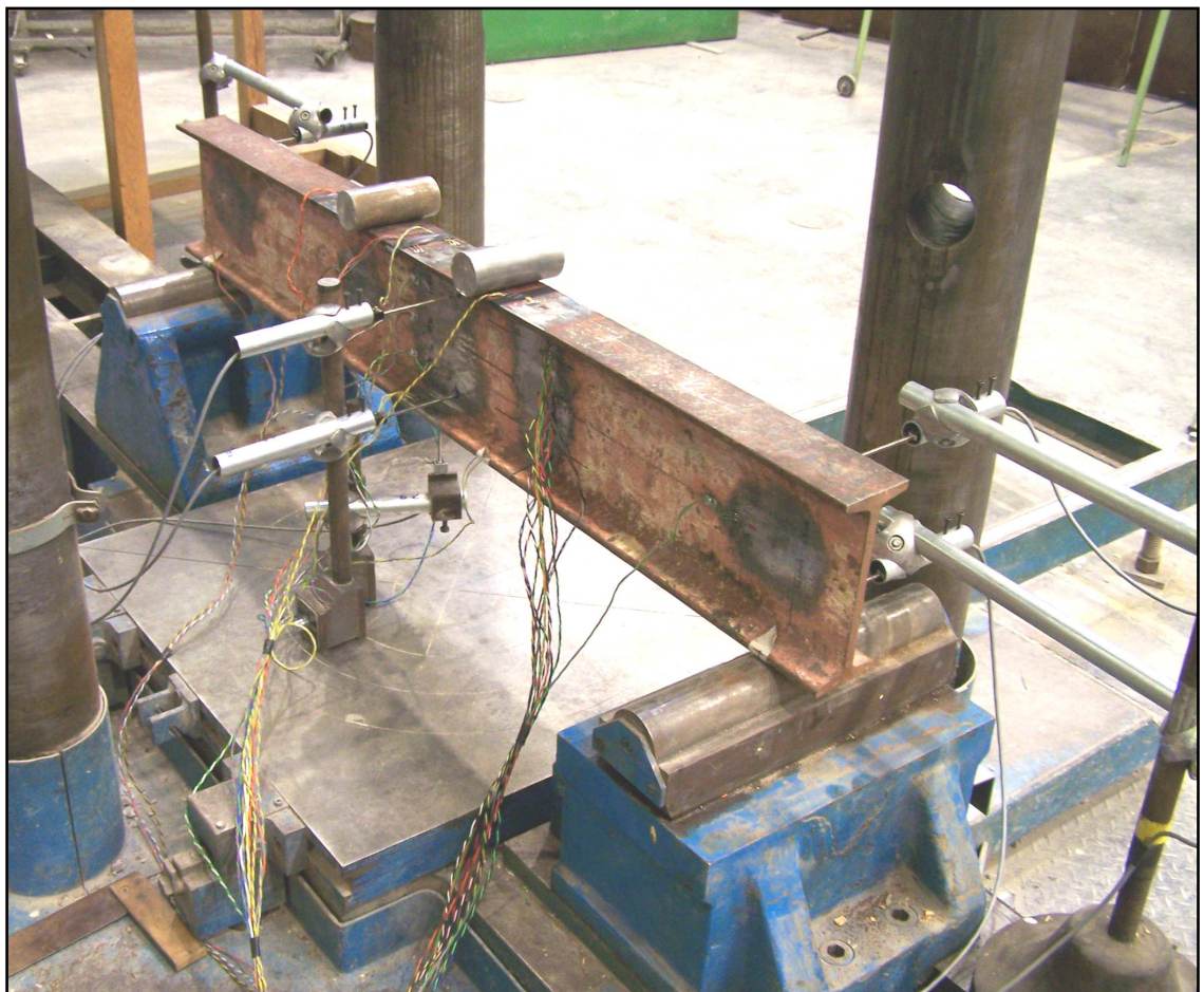
Figure 3.6 Loading and gauge arrangement for Albert Hall beam test. This picture shows the back elevation of the beam and can be compared directly with Figure 3.7. (Photo by M.O'Sullivan 2008)
