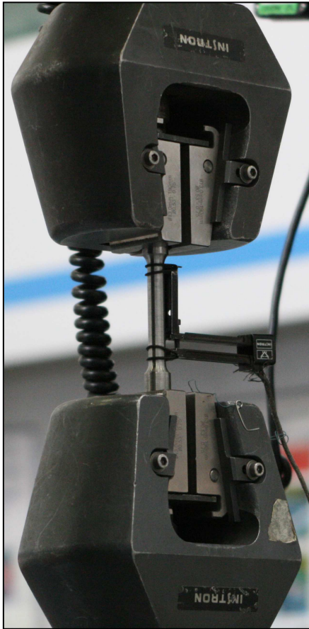
Figure 4.5 Test arrangement for round specimen
