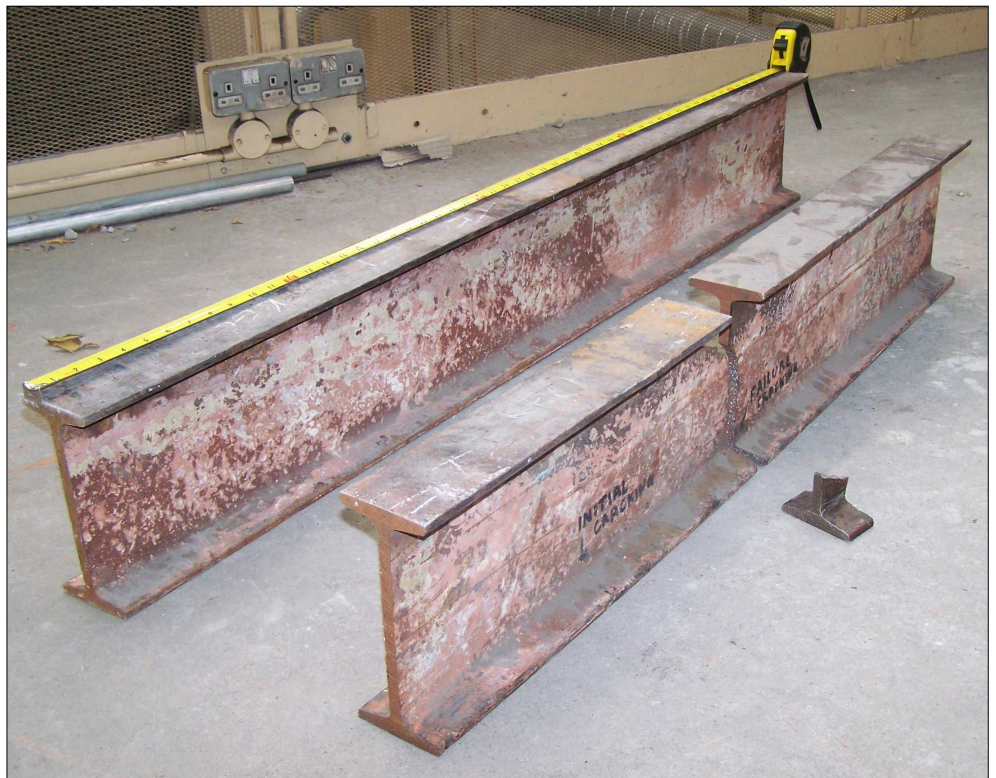
Figure 3.1 Rolled beam segments from Royal Albert Hall (Photo by M.O'Sullivan 2008)
