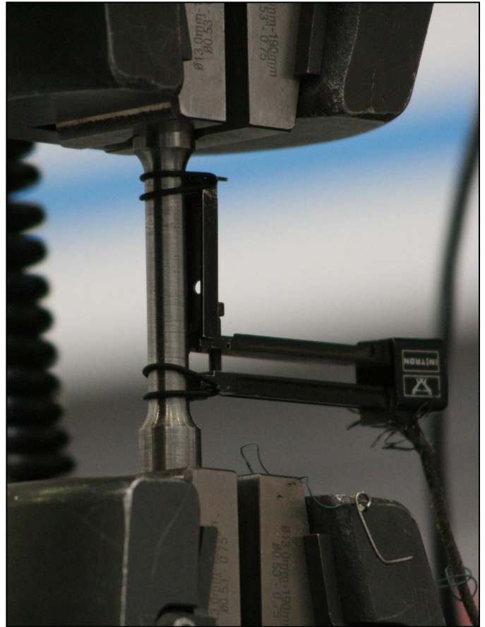
Figure 4.6 Close-up of test piece showing extensometer attached
