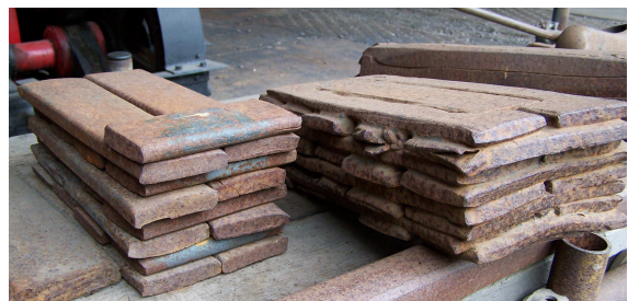
Figure 1.13 Cross-piling of wrought iron bars. (M.O'Sullivan 2008)
