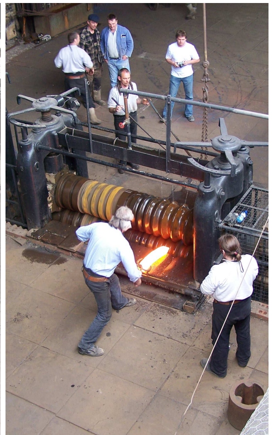
Figure 1.7 Inserting the billet for the first rolling (Photos by M.O'Sullivan at iron works of Blists Hill Victorian Town, Ironbridge Gorge, Shropshire 2008)
