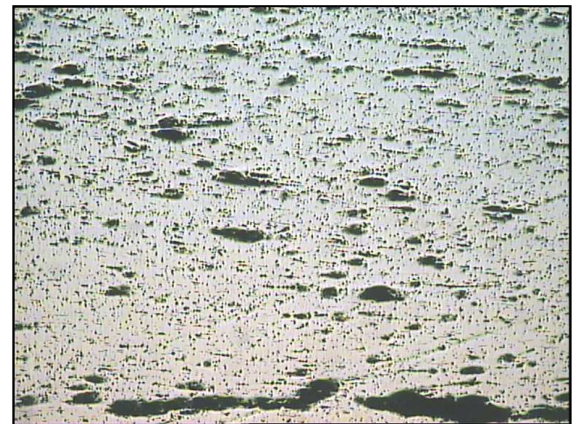
Figure 4.17 Plate iron under x5 magnification (Photo by M.O'Sullivan 2009)
