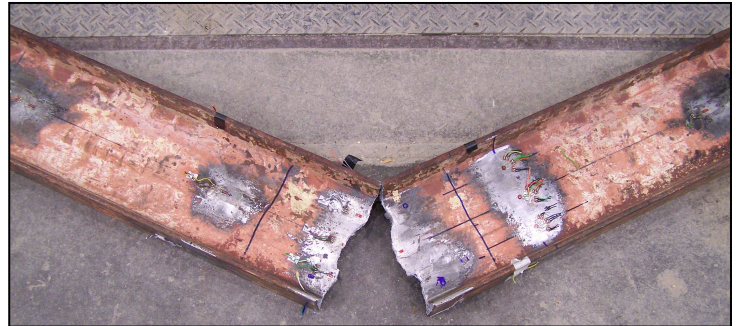
Figure 3.23 Broken beam after removal from testing machine (Photo by M.O'Sullivan 2008)
