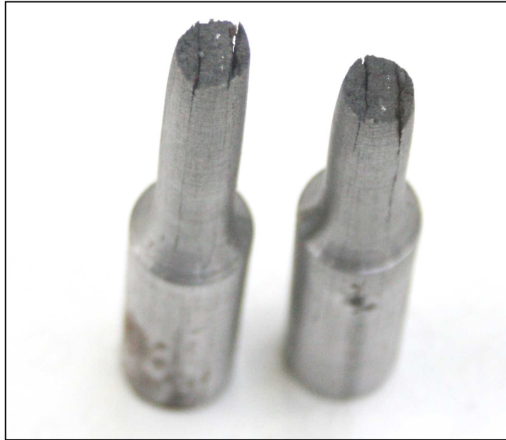
Figure 4.13 Test piece with longitudinal splits. (Photo by M.O'Sullivan 2009)
