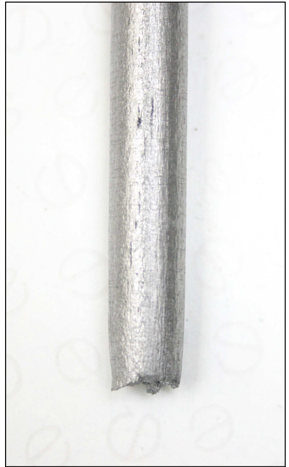
Figure 4.14 Stretching the test piece caused radial contraction across the section, and circumferential contraction of the metal surface, which gave it a rough texture. (M.O'Sullivan 2009)
