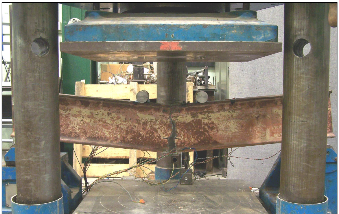
Figure 3.18 Notched beam at end of test showing crack through almost entire mid-span section. (Photo by M.O'Sullivan 2008)
