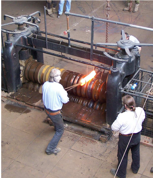
Figure 1.8 Passing the bar back (a dead pass) (Photos by M.O'Sullivan at iron works of Blists Hill Victorian Town, Ironbridge Gorge, Shropshire 2008)
