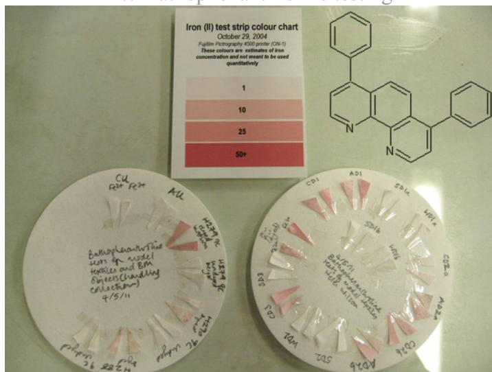
Figure 2.8 The bathophenanthroline test strips used to identify soluble iron(II) and iron(III) ions (using 1% aqueous ascorbic acid solution) on a variety of model and historic textiles as well as the semi-quantitative colour chart (Vuori and Tse 2005a) and the structure of bathophenanthroline
