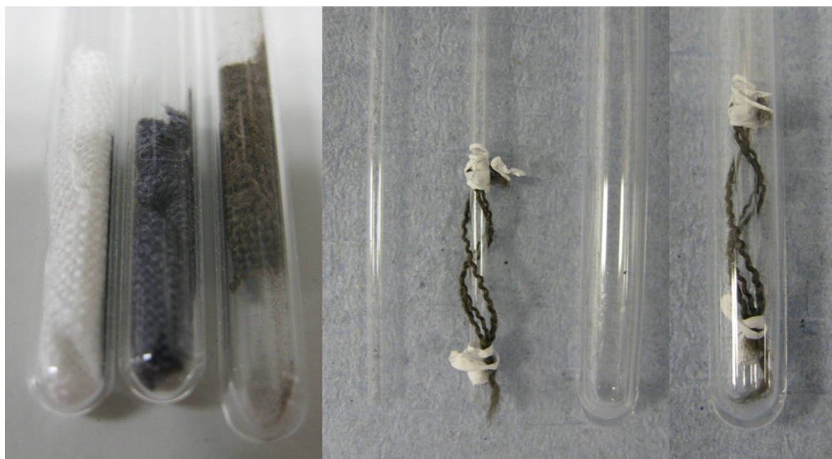
Figure 5.2 Undyed and dyed (unaged and aged) cotton samples prepared for qualitative analysis (left) and a sample of dyed wool (pictured on the right with the components required for the preparation) prepared using the newly developed method for quantitative analysis
