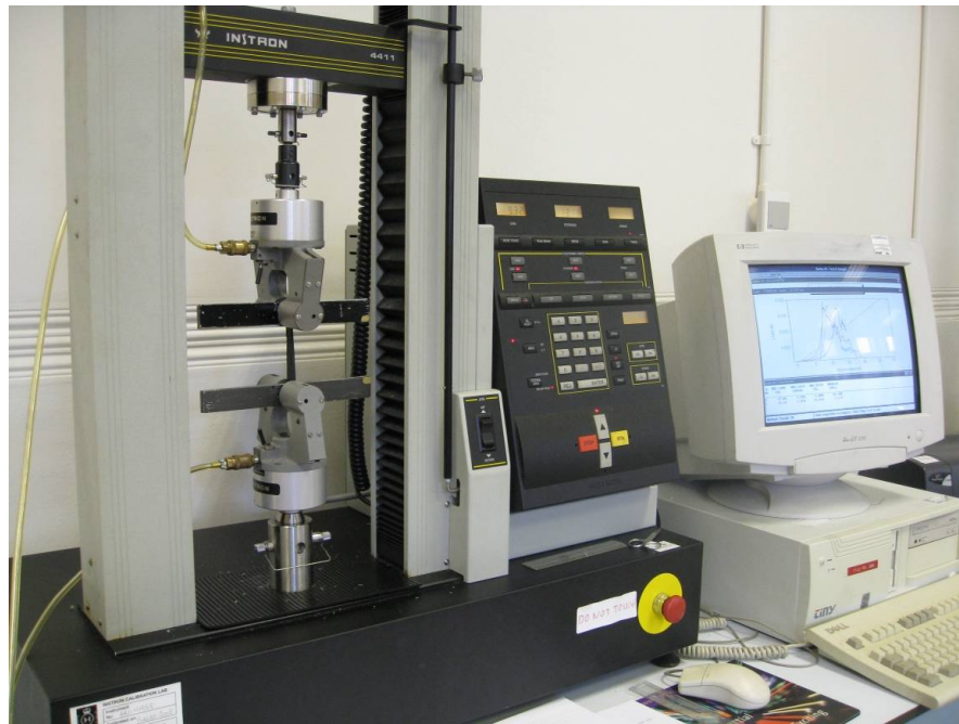
Figure 2.10 Photograph of the Instron 4411 tensile tester at the University of Manchester testing an aged dyed silk sample
