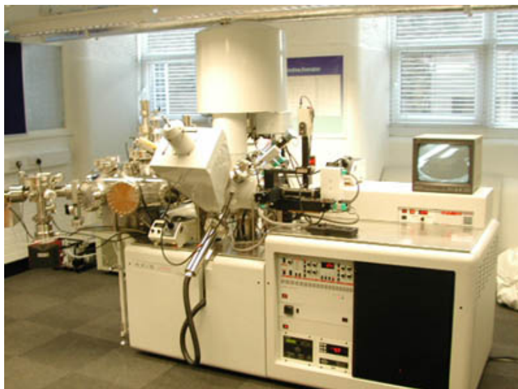
Fig. 2.22: A typical commercial XPS instrument (Kratos Axis Ultra) at Manchester University, showing the instrument X-ray sources and monochromator (center), electron analyser (top) and vacuum and pressure and control systems (left).
